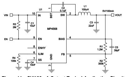
Figure 11 – 5V/100mA Output Typical Application Circuit
