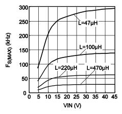
Figure 3 –  $f_{s(max)}$  at  $V_{OUT}=3.3V$
