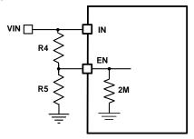
Figure 5 – Adjustable UVLO using EN pin
