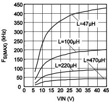
Figure 4 –  $f_{s(max)}$  at  $V_{OUT}=5V$
