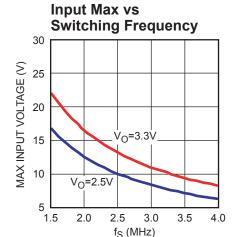
Figure 2—Recommended Input vs. fs
