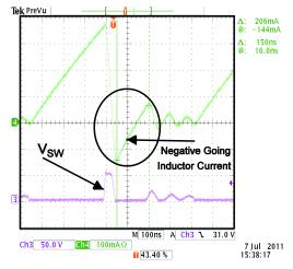
Due to the applied high-output voltage on the switch node combined with the  $C_{DS}$  capacitive coupling of the MP3430 FET, a significant reverse current flows through the inductor during the  $D_3$  period.
