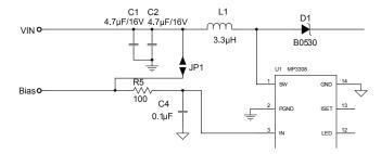
Figure 3—Input Bias Filtering
