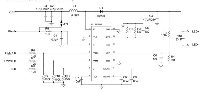
Figure 2—Typical Application Driving 9 Strings of 3 WLEDs
