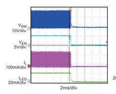
**PWM Dimming** f<sub>PWM</sub> = 200Hz, D = 50%
