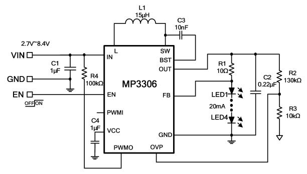
Figure 5— 4 LEDs in Series 20mA
