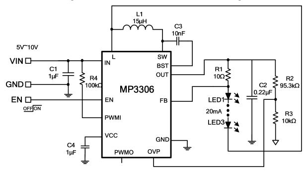
Figure 7— 3 LEDs in Series 20mA with 5~10V Input Voltage
