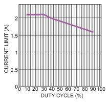
Figure 3—Current Limit Curve
