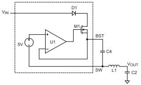
Figure 3: Internal Bootstrap Charging Circuit
