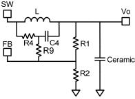
Figure 11: Simplified Circuit with Ceramic Capacitor
