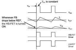
Figure 2: Heavy-Load Operation
