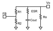
Figure 9: Simplified Circuit in Skip Mode
