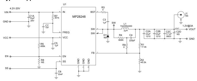
Figure 13: Detailed Application Schematic
