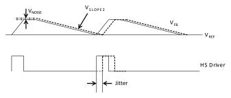
Figure 6: Jitter in Skip Mode
