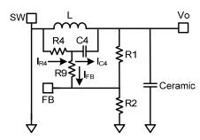
Figure 8: Simplified Circuit in PWM Mode with External Ramp Compensation
