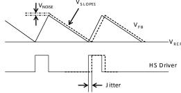
Figure 5: Jitter in PWM Mode
