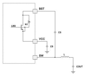
Figure 4: Floating Driver and Bootstrap Charging
