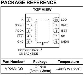
For Tape & Reel, add suffix –Z (eg. MP2631DQ–Z) For RoHS compliant packaging, add suffix –LF (eg. MP2631DQ–LF–Z)
