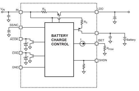
Figure 1—Functional Block Diagram
