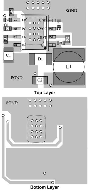
Figure 4—PCB Layout for Double Layers
