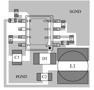
Figure 3—PCB Layout for Single Layer
