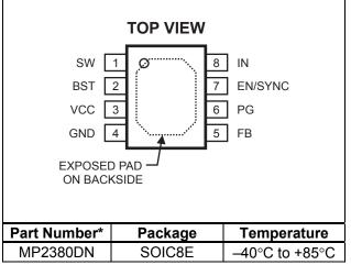
\* For Tape & Reel, add suffix –Z (e.g. MP2380DN–Z) For RoHS Compliant Packaging, add suffix –LF (e.g. MP2380DN–LF–Z)
