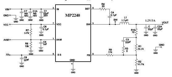
Figure 8: 12V<sub>IN</sub>, 1.2V/3A Output
