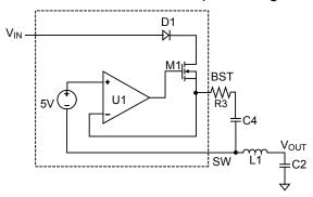
Figure 2: Internal Bootstrap Charging Circuit
