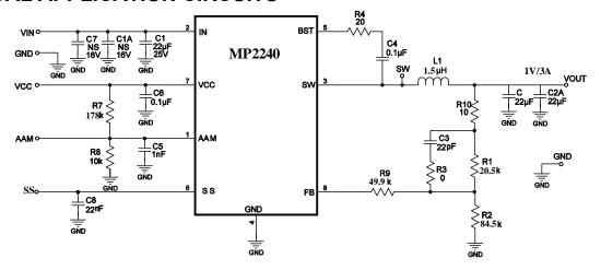
Figure 7: 12V<sub>IN</sub>, 1V/3A Output
