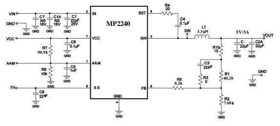
Figure 12: 12V<sub>IN</sub>, 5V/3A Output
