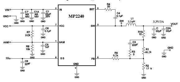
Figure 11: 12V<sub>IN</sub>, 3.3V/3A Output
