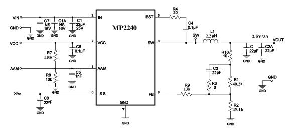
Figure 10: 12V<sub>IN</sub>, 2.5V/3A Output
