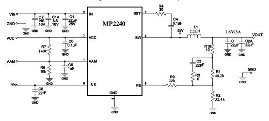
Figure 9: 12V<sub>IN</sub>, 1.8V/3A Output
