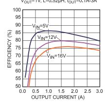
**Efficiency vs. Output Current**  $V_{OUT}$ =1.2V, L=0.52µH,  $I_{OUT}$ =0.1A-3A
