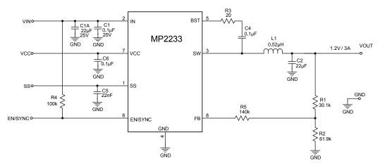
Figure 11: V<sub>IN</sub> = 12V, 1.2V/3A Output
