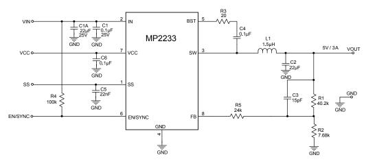
Figure 7:  $V_{IN} = 12V$ , 5V/3A Output
