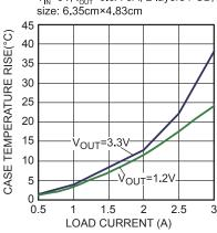
Case Temperature Rise vs. **Output Current**
