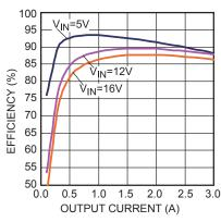
**Efficiency vs. Output Current** V<sub>OUT</sub>=3.3V, L=1.5μH, I<sub>OUT</sub>=0.1A-3A
