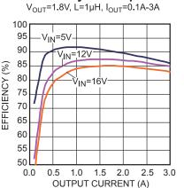
**Efficiency vs. Output Current**
