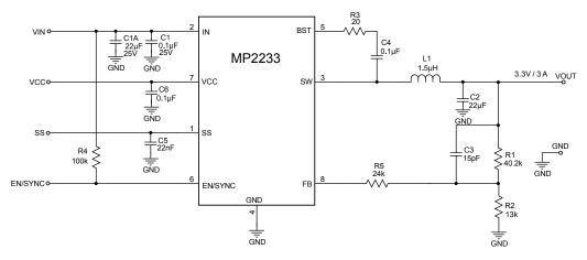
Figure 8:  $V_{IN}$  = 12V, 3.3V/3A Output
