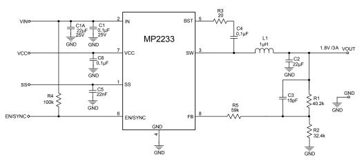
Figure 10:  $V_{IN}$  = 12V, 1.8V/3A Output
