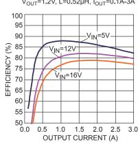
**Efficiency vs. Output Current**
