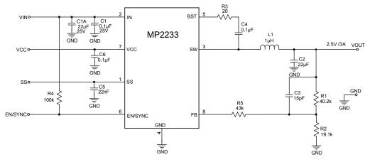
Figure 9: V<sub>IN</sub> = 12V, 2.5V/3A Output
