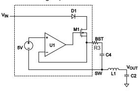
Figure 4: Internal Bootstrap Charging Circuit
