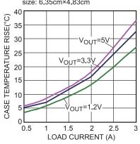
Case Temperature Rise vs. **Output Current**
