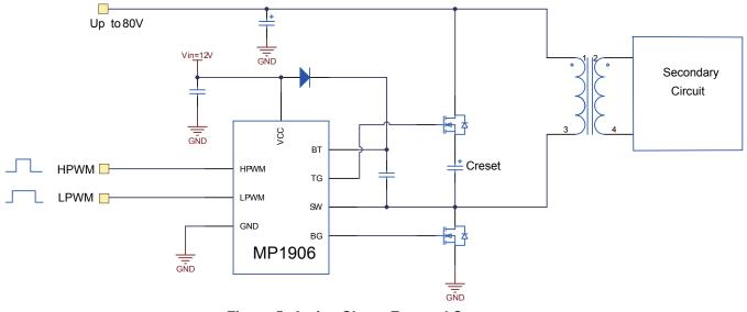
Figure 5: Active-Clamp Forward Converter
