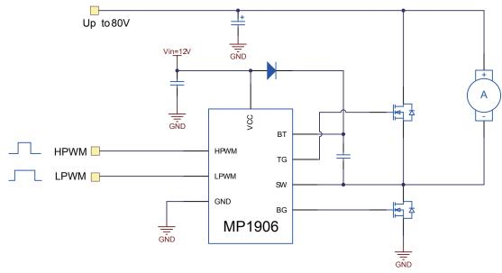
Figure 4: Half-Bridge Motor Driver
