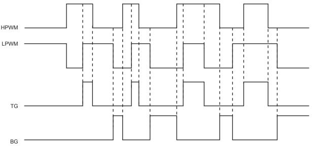
Figure 3: Input/Output Timing Diagram
