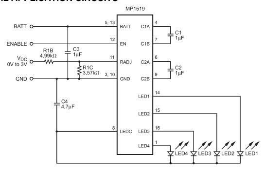
Figure 3—Analog Dimming Circuit
