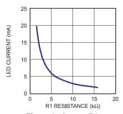
Figure 2—I<sub>LED</sub> vs. R1
