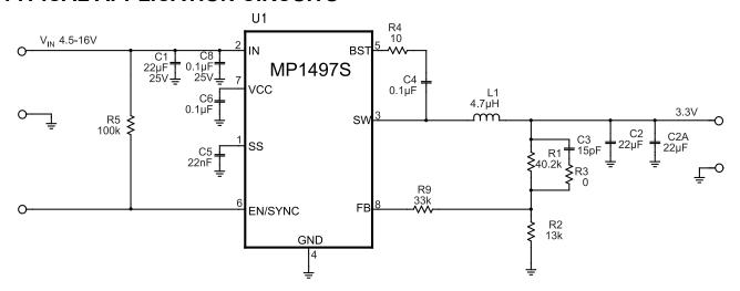
Figure 6: 12V<sub>IN</sub>, 3.3V/3A
