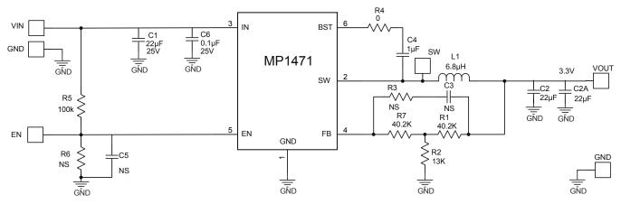
Figure 10: 12V<sub>IN</sub>, 3.3V/3A
