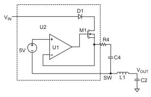
Figure 5 : Internal Bootstrap Charging Start-Up and Shutdown Circuit
