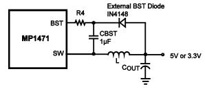
Figure 7 : Optional External Bootstrap Diode
