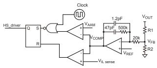
Figure 2: Simplified AAM Control Circuit
