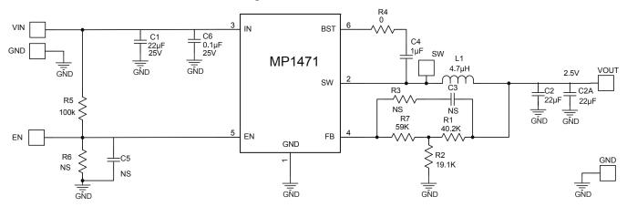
Figure 81: 12V<sub>IN</sub>, 2.5V/3A
