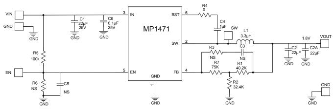
Figure 92: 12V<sub>IN</sub>, 1.8V/3A
