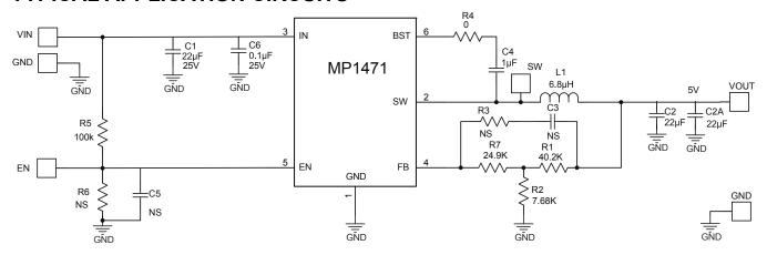
Figure 9: 12V<sub>IN</sub>, 5V/2.5A
