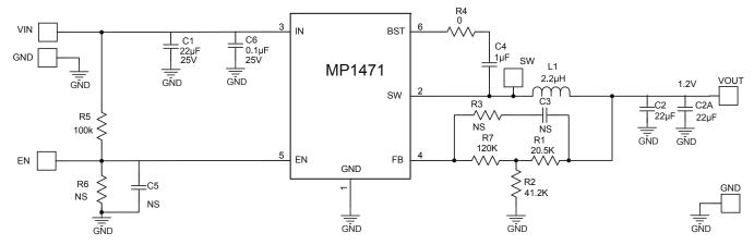
Figure 103: 12V<sub>IN</sub>, 1.2V/3A
