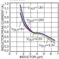
Figure 3: Inductor Peak Current vs. Inductor Value
