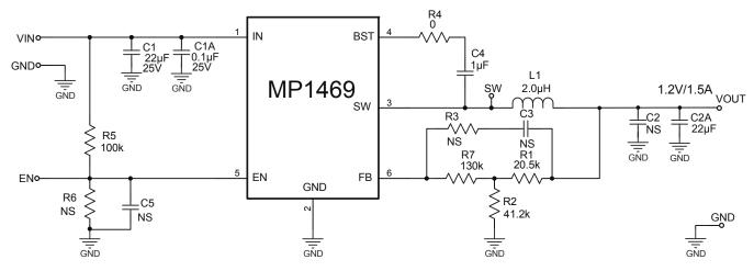
Figure 12: 12V<sub>IN</sub>, 1.2V/1.5A
