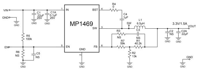
Figure 9: 12V<sub>IN</sub>, 3.3V/1.5A
