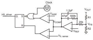
Figure 4—Simplified AAM Control Logic
