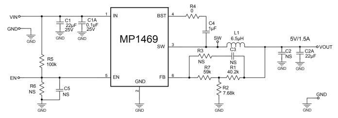
Figure 8: 12V<sub>IN</sub>, 5V/1.5A
