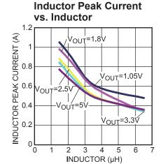
Figure5—Inductor Peak Current vs. Inductor
