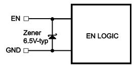
Figure 2: 6.5V Zener Diode Connection
