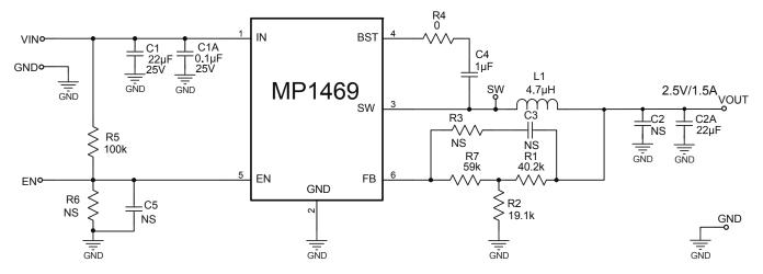
Figure 10: 12V<sub>IN</sub>, 2.5V/1.5A
