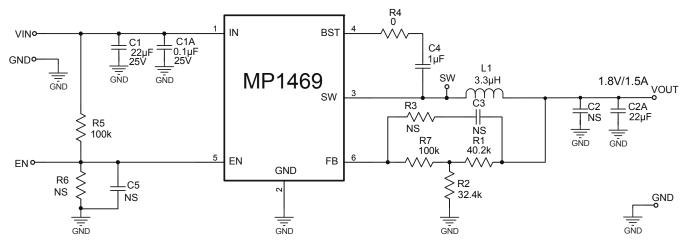
Figure 11: 12V<sub>IN</sub>, 1.8V/1.5A
