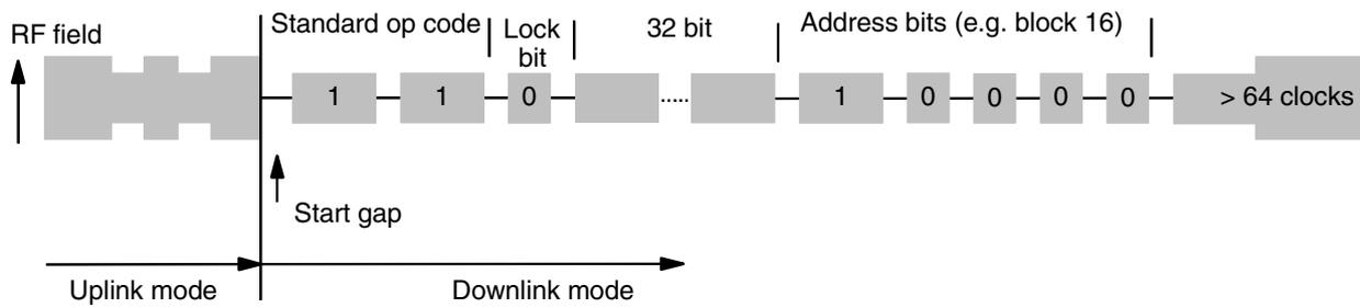
**Figure 9.** Explanation of the Programming Cycle
