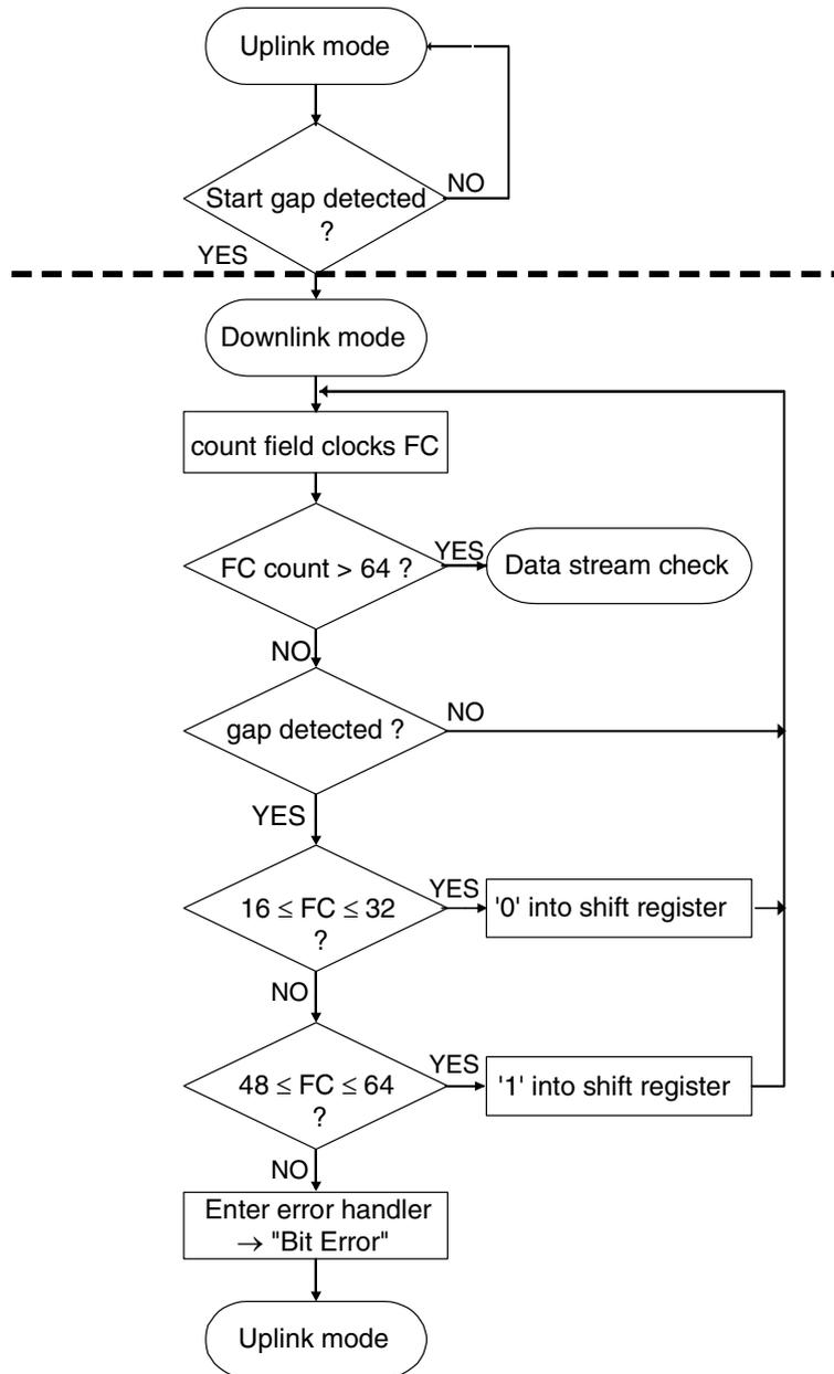
Figure 21. Data Stream Checking
