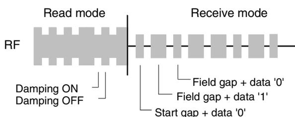
A start gap will be accepted at any time after start-up initialization has been finished (RF field ON plus  $\approx 1$  ms, start-up delay inactive) if the IC is not in downlink mode.
