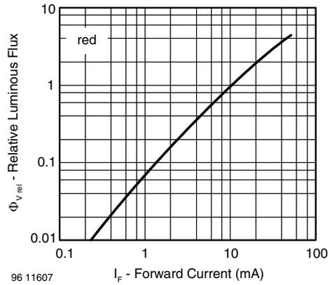
Fig. 6 - Relative Luminous Flux vs. Forward Current
