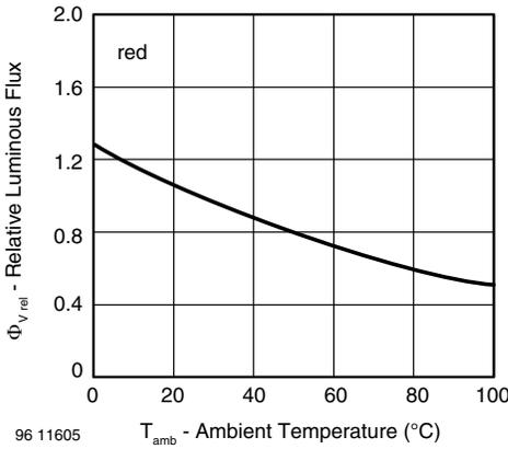
Fig. 4 - Relative Luminous Flux vs. Ambient Temperature
