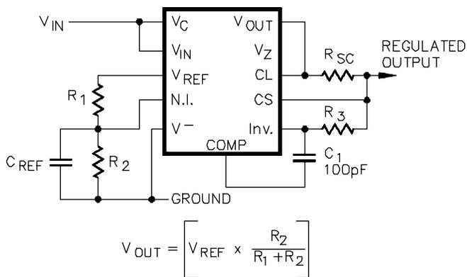
FIGURE 7 - BASIC LOW VOLTAGE REGULATOR
