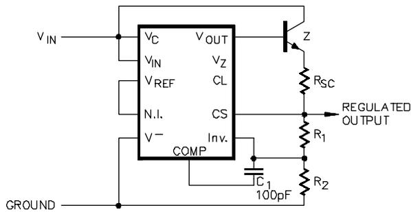
$$V_{OUT} = \left[ V_{REF} \times \frac{R_1 + R_2}{R_2} \right]$$
