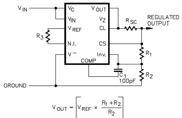
FIGURE 8 - BASIC HIGH VOLTAGE REGULATOR
