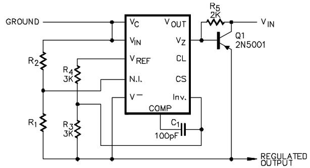
$$V_{OUT} = \left[ \frac{V_{REF}}{2} \times \frac{R_1 + R_2}{R_1} \right]; R_3 = R_4$$
