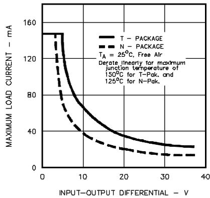
FIGURE 2. MAXIMUM LOAD CURRENT
