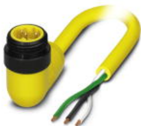
Power cable, 3-position, PVC, yellow, Plug angled 7/8"-16UNF, A - standard, on free cable end, cable length: 1 m
