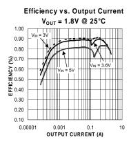
Figure 2. Efficiency Under Load
