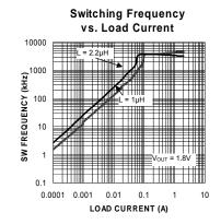
Figure 3. SW Frequency vs. Output Current
