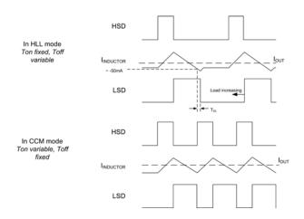
The diagram shows the signals for high side switch drive (HSD) for  $T_{ON}$  control, the inductor current and the low side switch drive (LSD) for  $T_{OFF}$  control.
