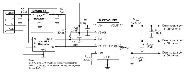
Figure 5. Multi-Port Bus-Powered Hub
