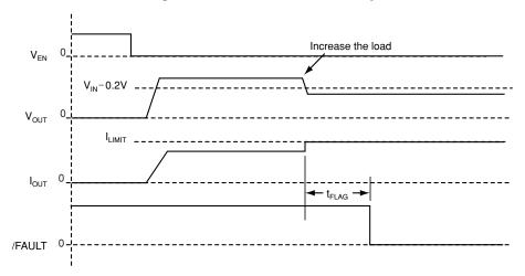
Figure 2. Overcurrent Fault Response — MIC2040-2
