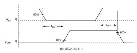
Figure 1. Turn-On/Turn-Off Delay
