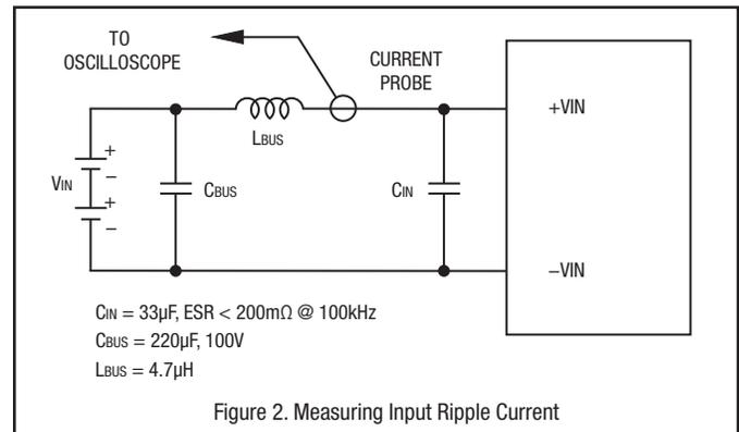
system configuration may require additional considerations. Please note that the values of  $C_{in}$ ,  $L_{bus}$  and  $C_{bus}$  may vary according to the specific converter model.
