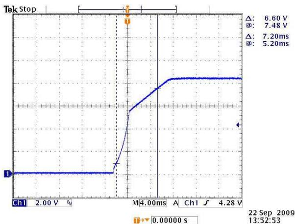
Power On Startup Output Delay
