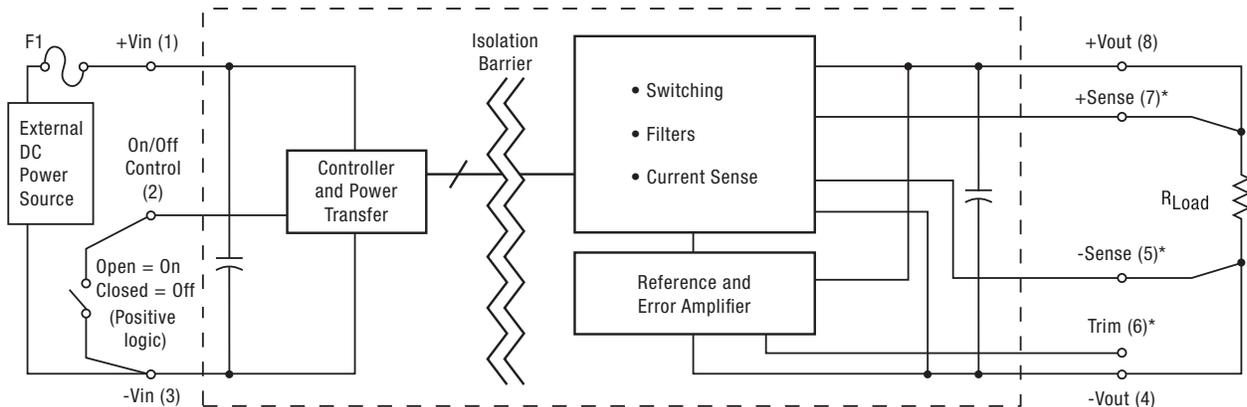
Figure 1. Connection Diagram
