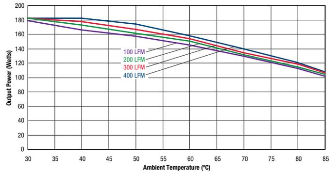
Maximum Power Temperature Derating vs. Airflow
