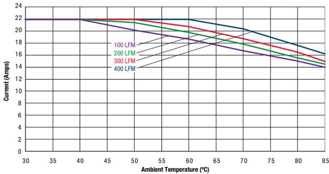
Maximum Current Temperature Derating vs. Airflow
