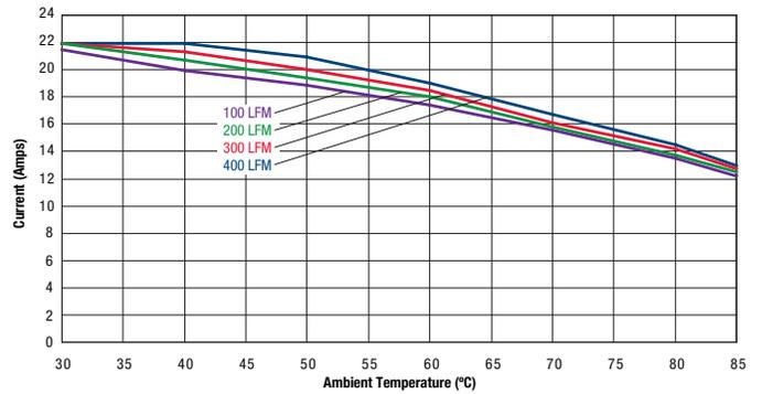
Maximum Current Temperature Derating vs. Airflow
