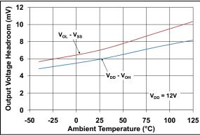
**FIGURE 2-27:** Output Voltage Headroom vs. Ambient Temperature.
