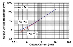
**FIGURE 2-25:** Output Voltage Headroom vs. Output Current.
