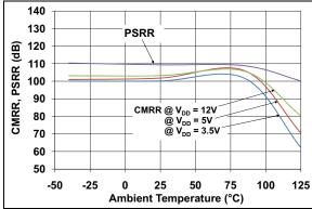
**FIGURE 2-11:** CMRR, PSRR vs. Ambient Temperature.
