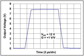
FIGURE 2-34: Large Signal Non-Inverting Pulse Response.
