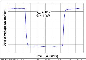
FIGURE 2-33: Small Signal Inverting Pulse Response.
