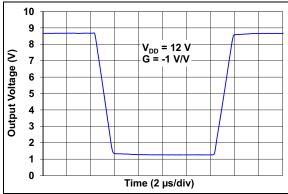
**FIGURE 2-35:** Large Signal Inverting Pulse Response.
