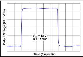
FIGURE 2-32: Small Signal Non-Inverting Pulse Response.
