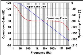
FIGURE 2-16: Open-Loop Gain, Phase vs. Frequency.
