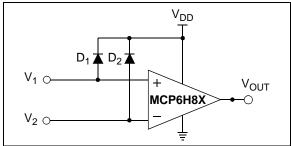
FIGURE 4-2: Protecting the Analog Inputs.
