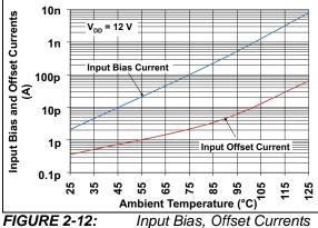
**FIGURE 2-12:** Input Bias, Offset Currents vs. Ambient Temperature.
