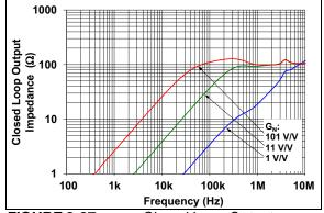
FIGURE 2-37: Closed Loop Output Impedance vs. Frequency.
