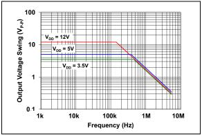
FIGURE 2-23: Output Voltage Swing vs. Frequency.
