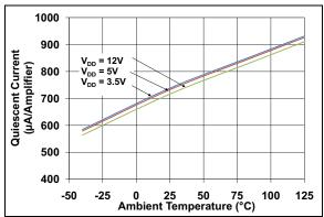
**FIGURE 2-14:** Quiescent Current vs. Ambient Temperature.
