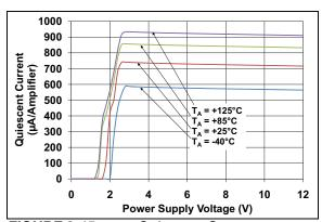
**FIGURE 2-15:** Quiescent Current vs. Power Supply Voltage.
