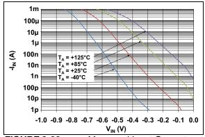
**FIGURE 2-38:** Measured Input Current vs. Input Voltage (below V<sub>SS</sub>).
