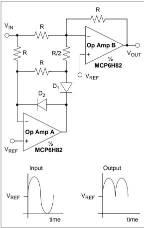
FIGURE 4-9: Active Full-Wave Rectifier.
