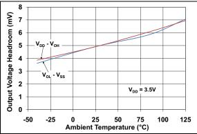
FIGURE 2-29: Output Voltage Headroom vs. Ambient Temperature.
