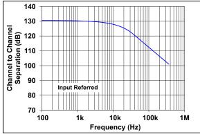
FIGURE 2-19: Channel-to-Channel Separation vs. Frequency (MCP6H82/4 only).
