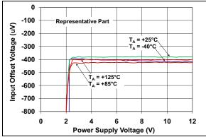
FIGURE 2-7: Input Offset Voltage vs. Power Supply Voltage.
