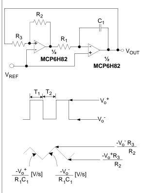
FIGURE 4-10: Triangle Waves Generator.
