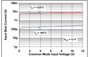
FIGURE 2-13: Input Bias Current vs. Common Mode Input Voltage.
