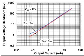
FIGURE 2-24: Output Voltage Headroom vs. Output Current.
