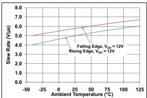
FIGURE 2-30: Slew Rate vs. Ambient Temperature.
