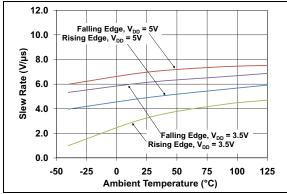
FIGURE 2-31: Slew Rate vs. Ambient Temperature.
