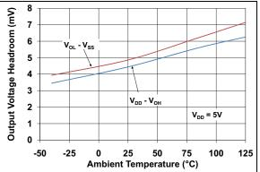
**FIGURE 2-28:** Output Voltage Headroom vs. Ambient Temperature.
