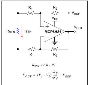
FIGURE 4-8: High Side Current Sensing Using Difference Amplifier.
