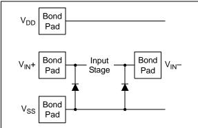
FIGURE 4-1: Simplified Analog Input ESD Structures.
