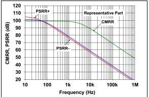
**FIGURE 2-10:** CMRR, PSRR vs. Frequency.
