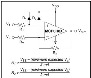
FIGURE 4-3: Protecting the Analog Inputs.
