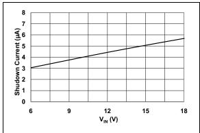
FIGURE 2-19: Shutdown Current vs. Input Voltage.
