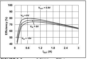
FIGURE 2-6: 0.9V V<sub>OUT</sub> Efficiency vs. I<sub>OUT</sub>.
