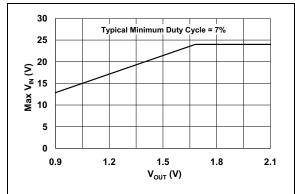
**FIGURE 2-25:** Maximum V<sub>IN</sub> to V<sub>OUT</sub> Ratio for Continuous Switching.
