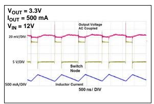
FIGURE 2-27: Heavy Load Switching Waveforms.
