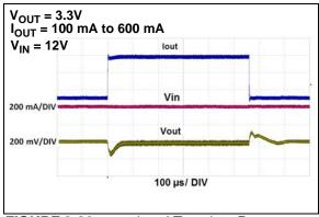
FIGURE 2-30: Load Transient Response.
