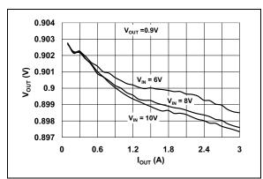
**FIGURE 2-12:** 0.9V V<sub>OUT</sub> vs. I<sub>OUT</sub>.
