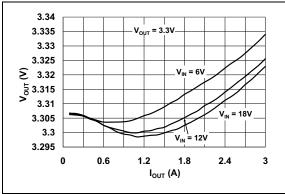
**FIGURE 2-8:** 3.3V V<sub>OUT</sub> vs. I<sub>OUT</sub>.
