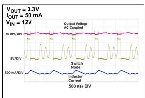
FIGURE 2-26: Light Load Switching Waveforms.
