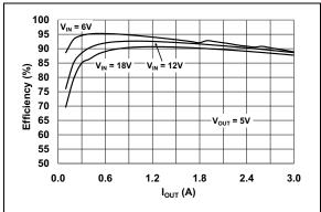
FIGURE 2-1: 5V V<sub>OUT</sub> Efficiency vs. I<sub>OUT</sub>.
