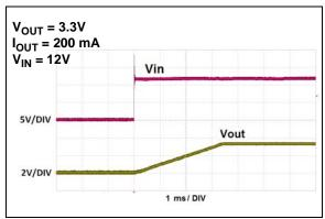
**FIGURE 2-29:** Start-up From  $V_{IN}$
