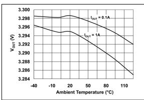
**FIGURE 2-21:** Output Voltage vs. Temperature.
