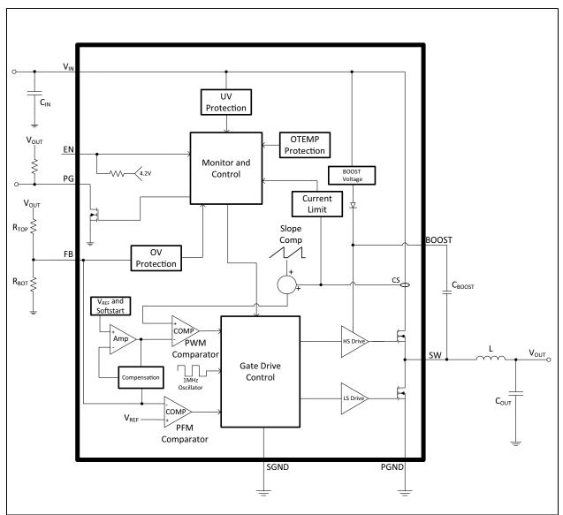
FIGURE 4-1: MCP16323 Block Diagram.
