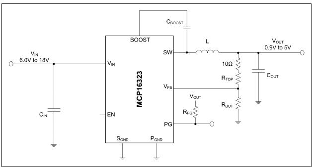
FIGURE 5-2: Recommended Layout – Schematic.
