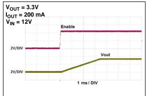
FIGURE 2-28: Start-up From Enable.
