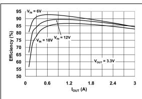
**FIGURE 2-2:** 3.3V V<sub>OUT</sub> Efficiency vs. I<sub>OUT</sub>.
