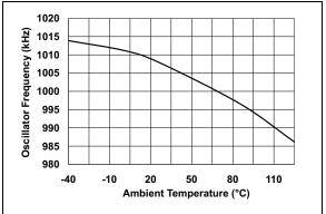
**FIGURE 2-22:** Oscillator Frequency vs. Temperature ( $I_{OUT} = 300 \text{ mA}$ ).
