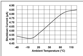
FIGURE 2-20: Shutdown Current vs. Temperature.
