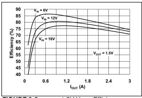
FIGURE 2-5: 1.5V V<sub>OUT</sub> Efficiency vs. I<sub>OUT</sub>.
