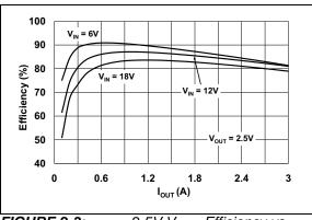
**FIGURE 2-3:** 2.5V  $V_{OUT}$  Efficiency vs.  $I_{OUT}$ .
