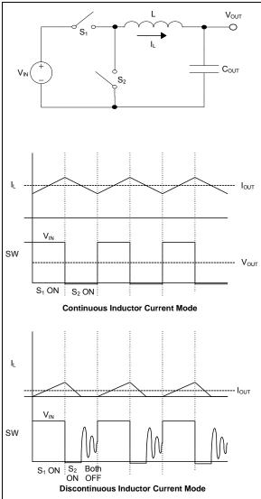
FIGURE 4-2: Synchronous Step-Down Converter.
