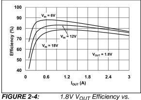
**FIGURE 2-4:** 1.8V  $V_{OUT}$  Efficiency vs.  $I_{OUT}$ .
