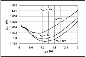
**FIGURE 2-10:** 1.8V V<sub>OUT</sub> vs. I<sub>OUT</sub>.
