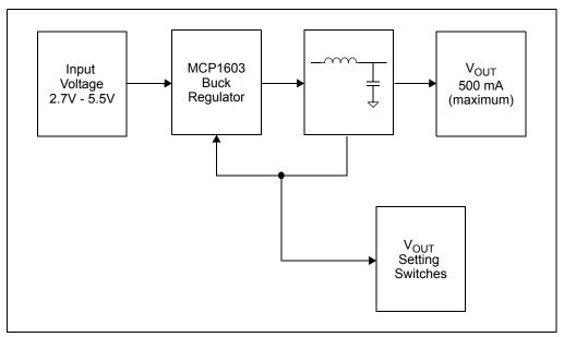
FIGURE 1-1: MCP1603 Buck Converter Evaluation Board Block Diagram.
