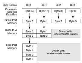
Figure 18-2. Connections for External Memory Port Sizes
