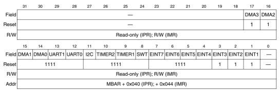
Figure 9-4. Interrupt Pending Register (IPR) and Interrupt Mask Register (IMR)
