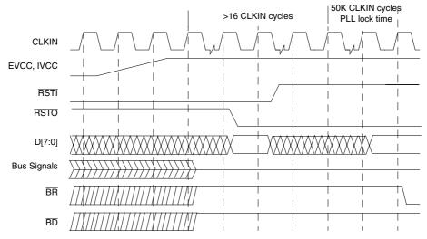
Figure 18-33. Master Reset Timing
