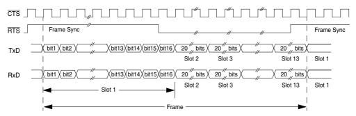
Figure 14-33. AC '97 Interface Timing
