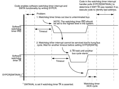
Figure 6-4. MCF5407 Embedded System Recovery from Unterminated Access
