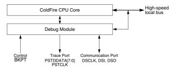
Figure 5-1. Processor/Debug Module Interface
