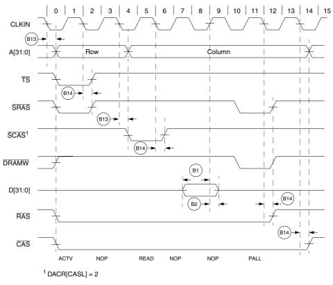
Figure 20-11. SDRAM Read Cycle with EDGESEL Tied Low
