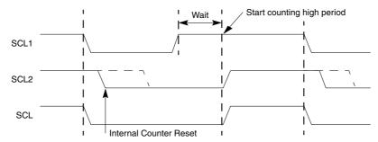
Figure 8-4. Synchronized Clock SCL
