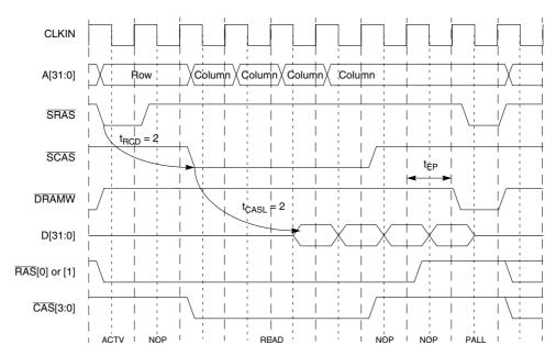
Figure 11-18. Burst Read SDRAM Access
