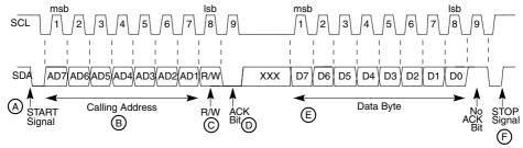
Figure 8-2. I<sup>2</sup>C Standard Communication Protocol
