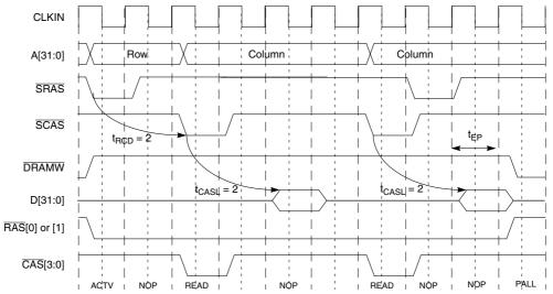
Figure 11-20. Synchronous, Continuous Page-Mode Access - Consecutive Reads
