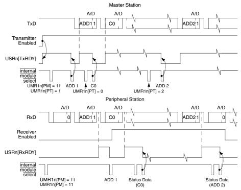
Figure 14-38. Multidrop Mode Timing Diagram
