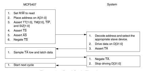
Figure 18-5. Read Cycle Flowchart
