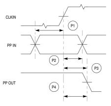
Figure 20-22. General-Purpose I/O Timing
