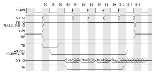
Figure 18-13. Line Read Burst (2-1-1-1), Internal Termination
