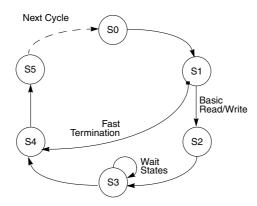
Figure 18-4. Data Transfer State Transition Diagram
