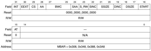
Figure 12-8. DMA Control Registers (DCRn)
