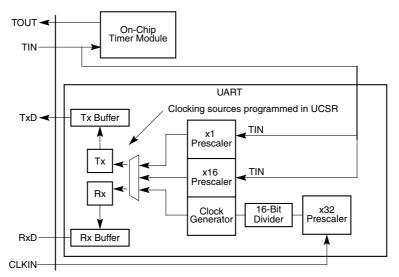
Figure 14-28. Clocking Source Diagram
