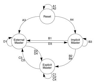
Figure 18-29. MCF5407 Two-Wire Bus Arbitration Protocol State Diagram
