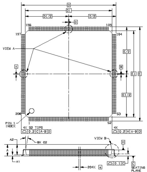
Figure 16-2. MCF5407 Case Drawing (General View)
