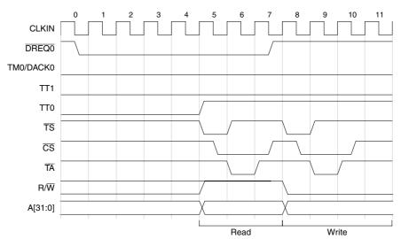
Figure 12-11. DREQ Timing Constraints, Dual-Address DMA Transfer
