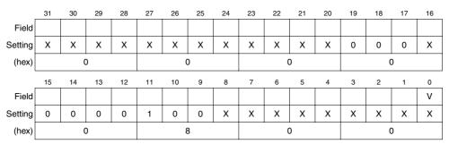
Figure 11-29. Mode Register Mapping to MCF5407 A[31:0]
