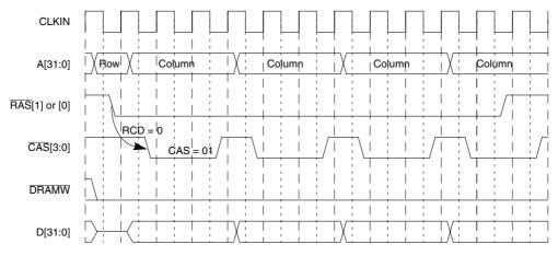
Figure 11-8. Burst Page-Mode Write Operation (4-3-3-3)
