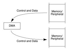
Figure 12-3. Dual-Address Transfer
