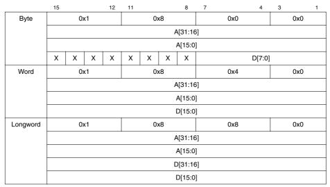
Figure 5-26. WRITE Command Format
