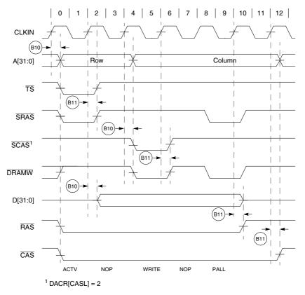
Figure 20-10. SDRAM Write Cycle with EDGESEL Tied High
