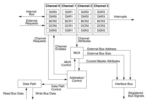
Figure 12-1. DMA Signal Diagram
