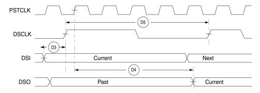
Figure 20-16. BDM Serial Port AC Timing
