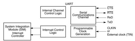
Figure 1-2. UART Module Block Diagram
