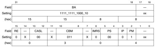
Figure 11-27. DACR Register Configuration
