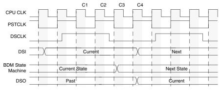
Figure 5-15. BDM Serial Interface Timing
