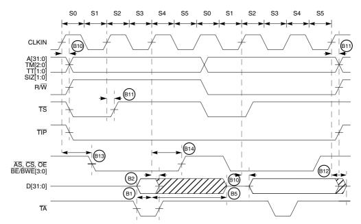
Figure 20-6. AC Timings—Normal Read and Write Bus Cycles
