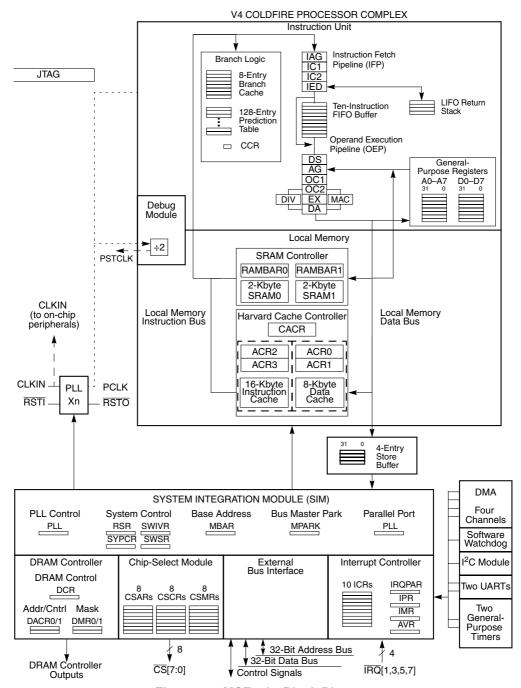
Figure 1-1. MCF5407 Block Diagram
