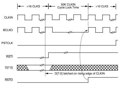
Figure 7-4. Reset and Initialization Timing
