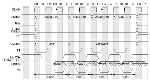
Figure 18-15. Line Read Burst-Inhibited, Fast, External Termination
