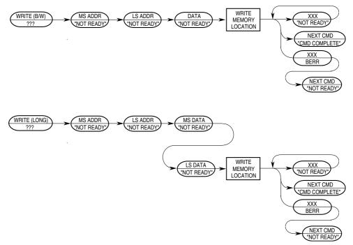
Figure 5-27. WRITE Command Sequence
