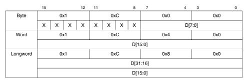
Figure 5-30. FILL Command Format
