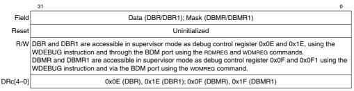
Figure 5-10. Data Breakpoint/Mask Registers (DBR/DBR1 and DBMR/DBMR1)
