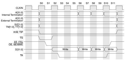
Figure 18-16. Line Write Burst (2-1-1-1), Internal/External Termination
