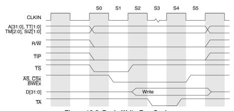
Figure 18-8. Basic Write Bus Cycle
