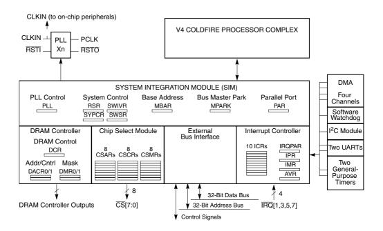
Figure 6-1. SIM Block Diagram
