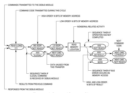
Figure 5-19. Command Sequence Diagram
