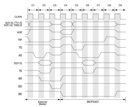
Figure 18-31. Three-Wire Bus Arbitration
