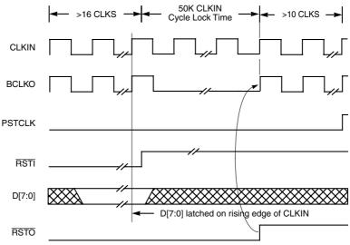
Figure 18-34. Software Watchdog Reset Timing
