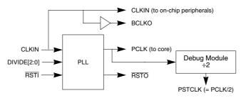
Figure 7-1. PLL Module Block Diagram
