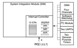
Figure 9-1. Interrupt Controller Block Diagram
