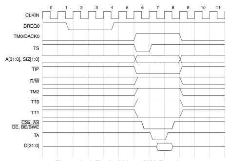
Figure 12-13. Single-Address DMA Transfer
