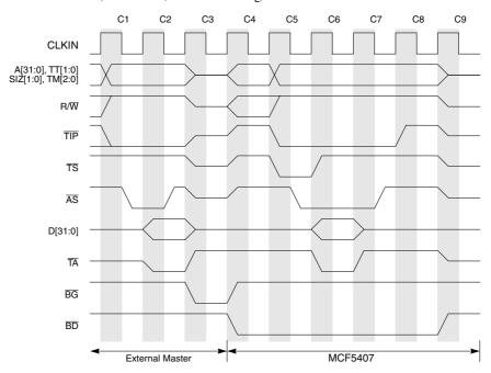
Figure 18-27. Two-Wire Bus Arbitration with Bus Request Asserted
