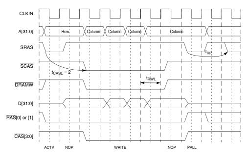
Figure 11-19. Burst Write SDRAM Access
