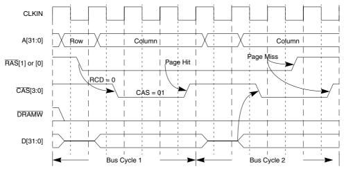
Figure 11-10. Write Hit in Continuous Page Mode
