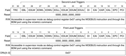
Figure 5-13. Trigger Definition Register (TDR)
