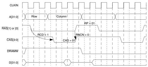
Figure 11-6. Basic Non-Page-Mode Operation RCD = 1, RNCN = 0 (5-5-5-5)
