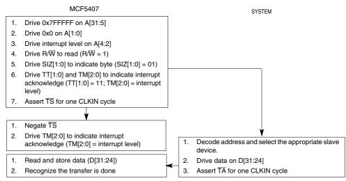
Figure 18-23. Interrupt-Acknowledge Cycle Flowchart
