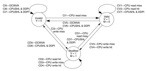
Figure 4-13. Data Cache Line State Diagram—Copyback Mode
