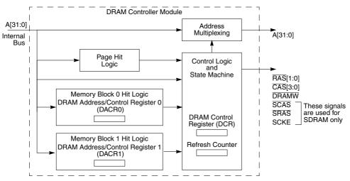
Figure 11-1. Asynchronous/Synchronous DRAM Controller Block Diagram
