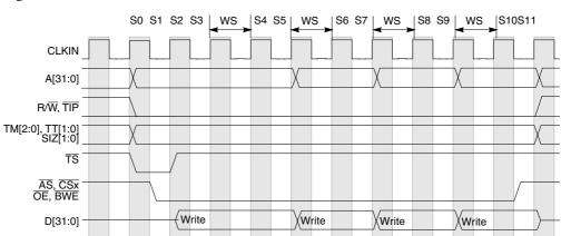
Figure 18-17 shows a line burst write with one wait-state insertion.
