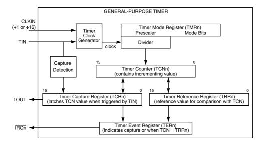
Figure 13-1. Timer Block Diagram
