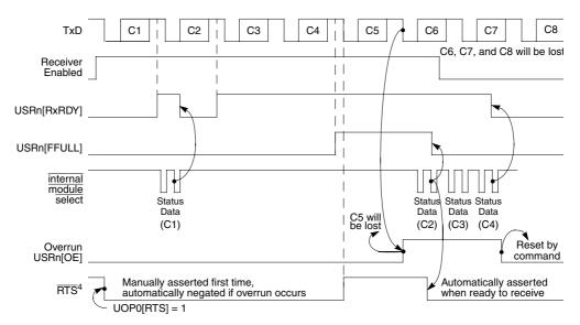
Figure 14-34. Receiver Timing
