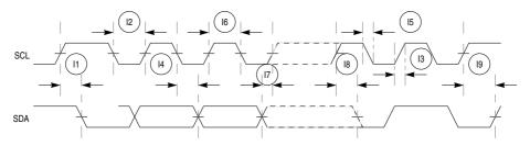
Figure 20-18. I<sup>2</sup>C Input/Output Timings
