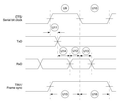
Figure 20-20. UART1 in 8- and 16-bit CODEC Mode
