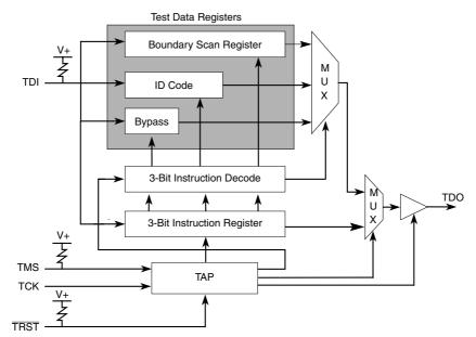
Figure 19-1. JTAG Test Logic Block Diagram
