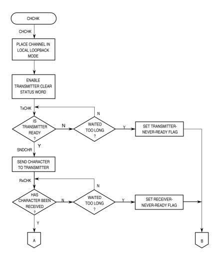
Figure 14-39. UART Mode Programming Flowchart (Sheet 2 of 5)
