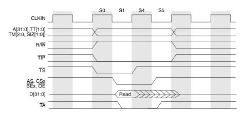
Figure 18-9. Read Cycle with Fast Termination
