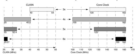
Figure 20-3. CLKIN-to-Core Clock Frequency Ranges
