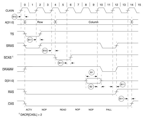
Figure 20-9. SDRAM Read Cycle with EDGESEL Tied High
