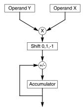
Figure 2-2. ColdFire Multiply-Accumulate Functionality Diagram
