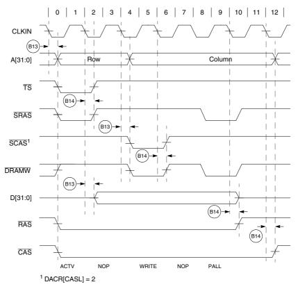
Figure 20-12. SDRAM Write Cycle with EDGESEL Tied Low
