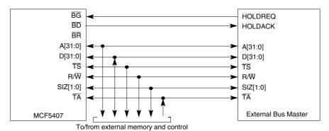
Figure 18-26. MCF5407 Two-Wire Mode Bus Arbitration Interface
