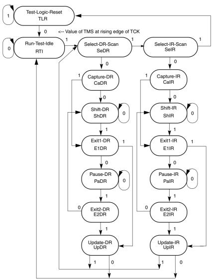
Figure 19-2. JTAG TAP Controller State Machine
