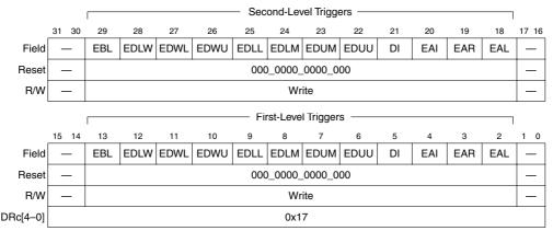
Figure 5-14. Extended Trigger Definition Register (XTDR)
