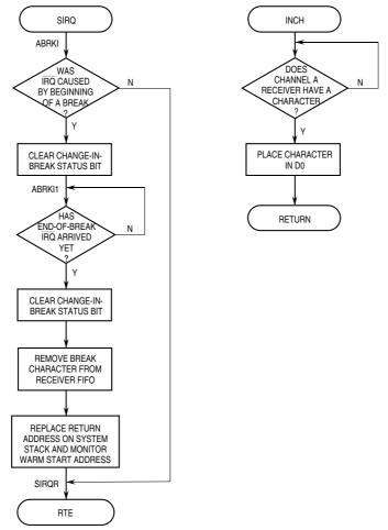
Figure 14-39. UART Mode Programming Flowchart (Sheet 4 of 5)
