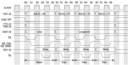
Figure 18-18. Line Write Burst-Inhibited, Internal Termination
