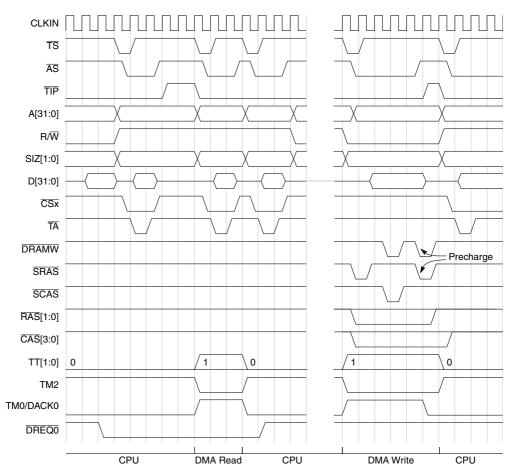
Figure 12-12. Dual-Address, Peripheral-to-SDRAM, Lower-Priority DMA Transfer
