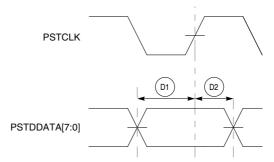
Figure 20-15. Real-Time Trace AC Timing
