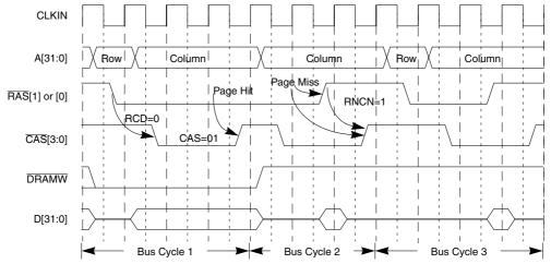
Figure 11-9. Continuous Page-Mode Operation
