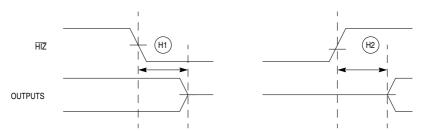
Figure 20-13. AC Output Timing—High Impedance
