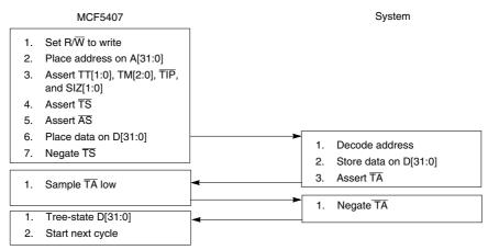
Figure 18-7. Write Cycle Flowchart
