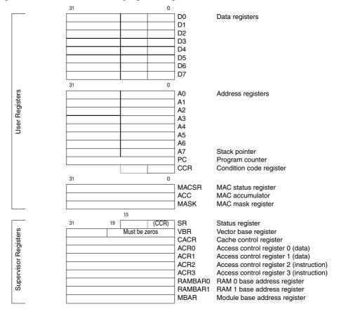
Figure 1-4. ColdFire MCF5407 Programming Model
