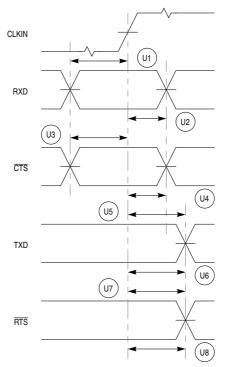
Figure 20-19. UART0 and UART1 Module AC Timing—UART Mode
