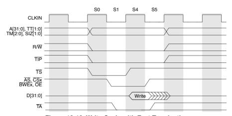
Figure 18-10. Write Cycle with Fast Termination
