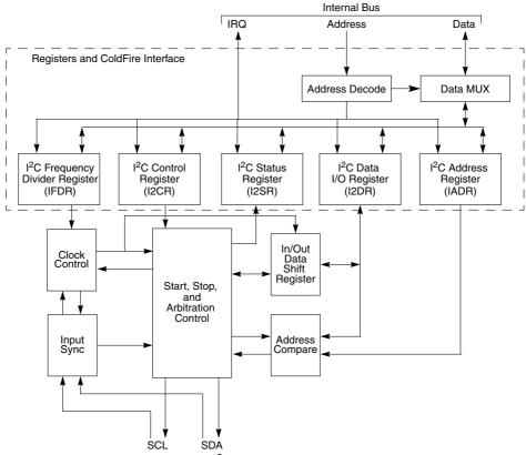
Figure 8-1. I<sup>2</sup>C Module Block Diagram
