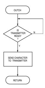
Figure 14-39. UART Mode Programming Flowchart (Sheet 5 of 5)
