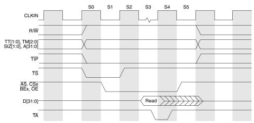
Figure 18-6. Basic Read Bus Cycle
