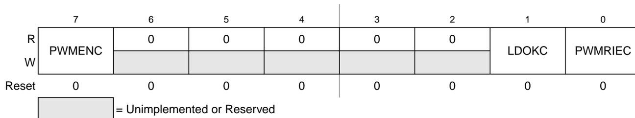
**Figure 11-36. PMF Enable Control C Register (PMFENCC)**
