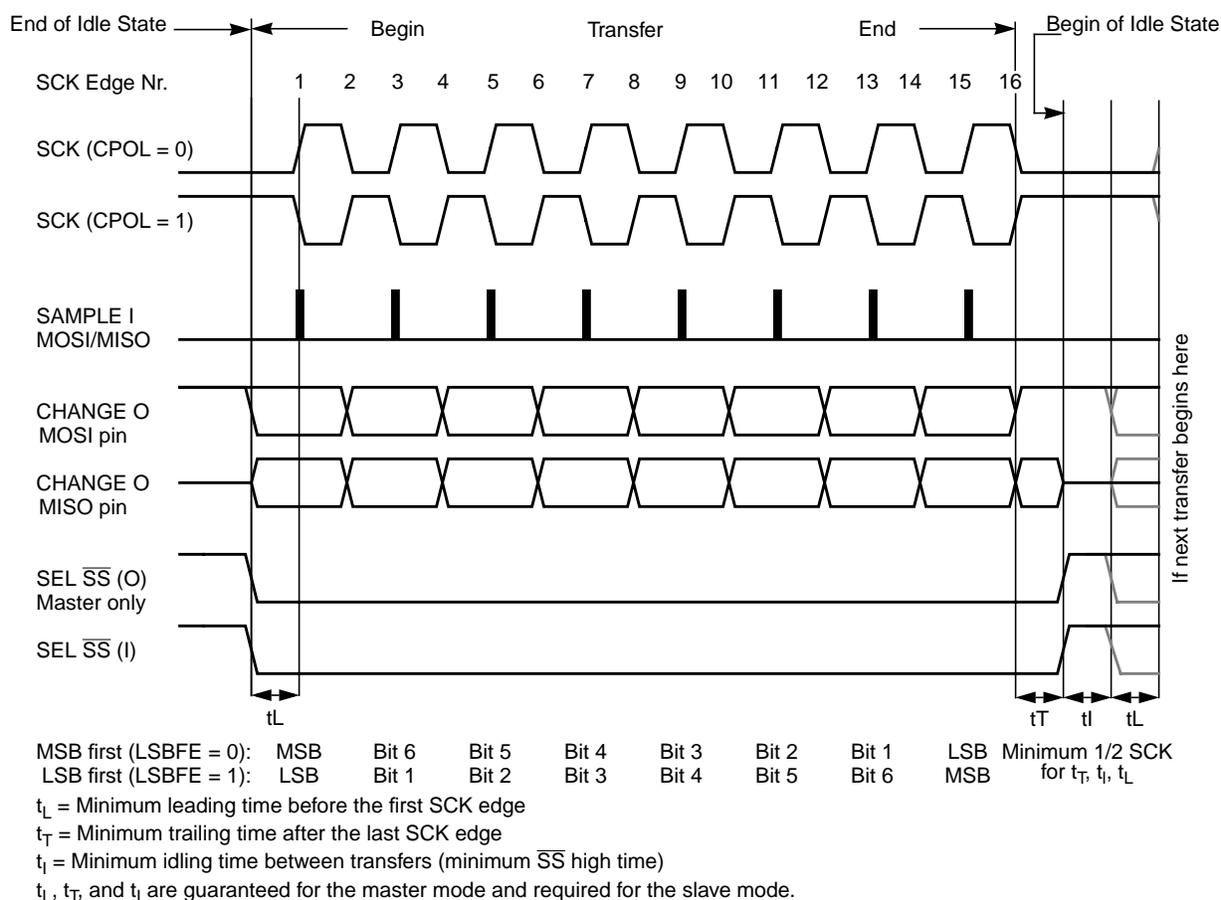
**Figure 9-9. SPI Clock Format 0 (CPHA = 0)**
