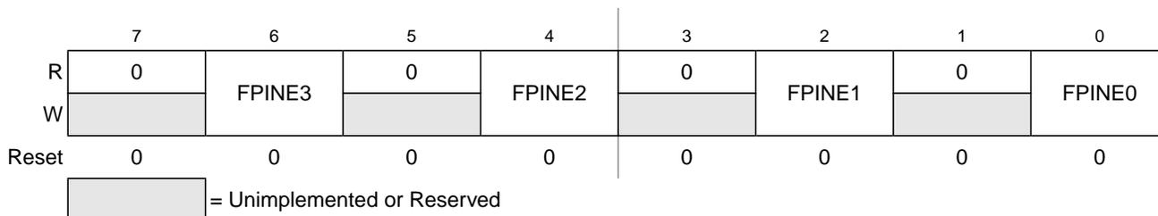
Figure 11-9. PMF Fault Pin Enable Register (PMFFPIN)
