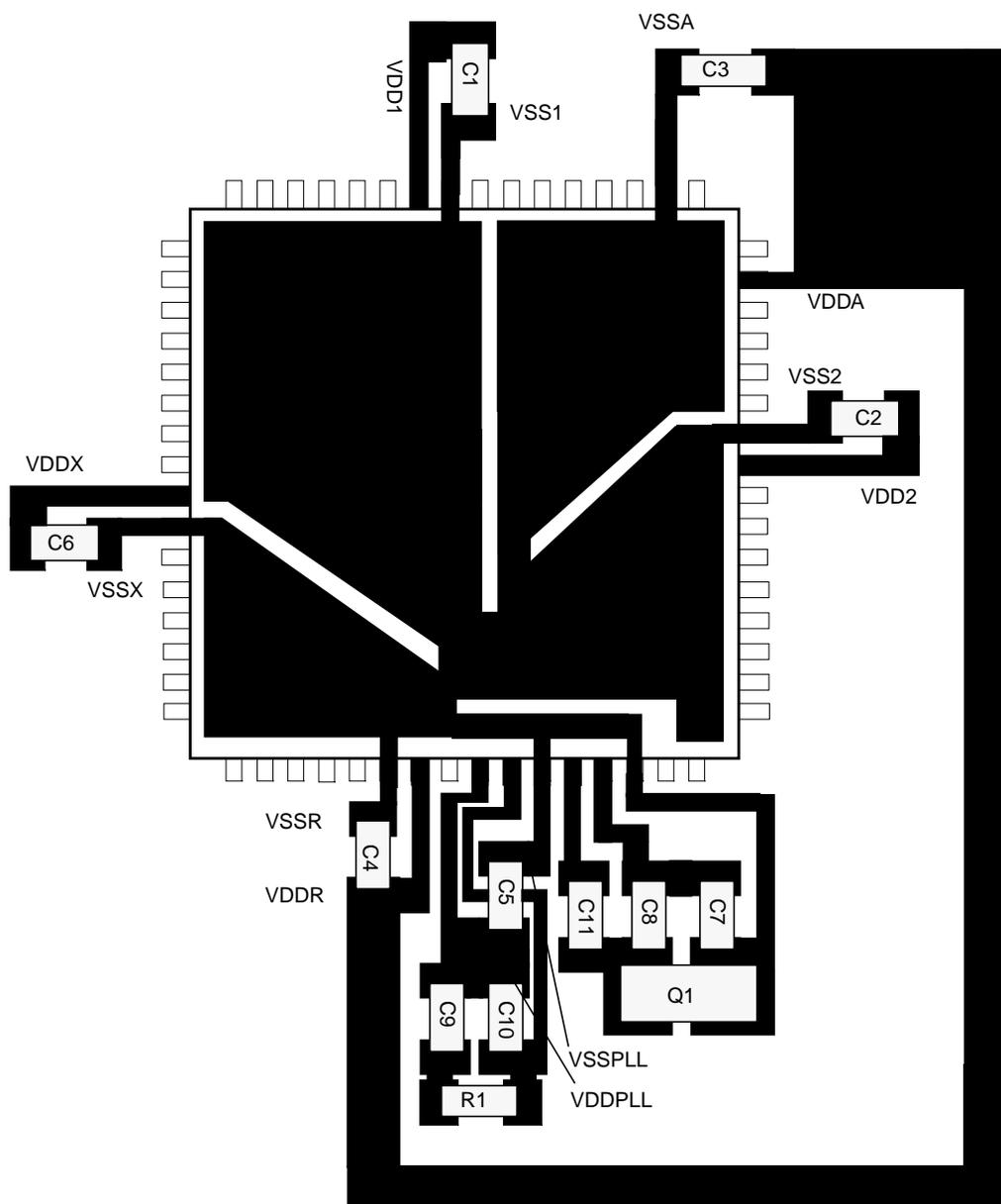
Figure 1-13. Recommended PCB Layout (64-QFN)
