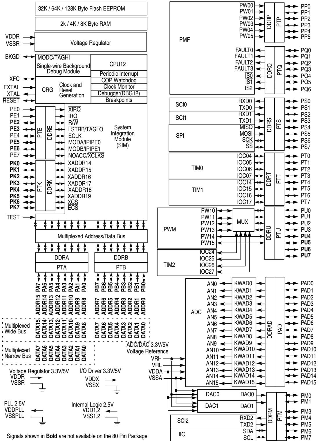
Figure 1-1. MC9S12E128 Block Diagram
