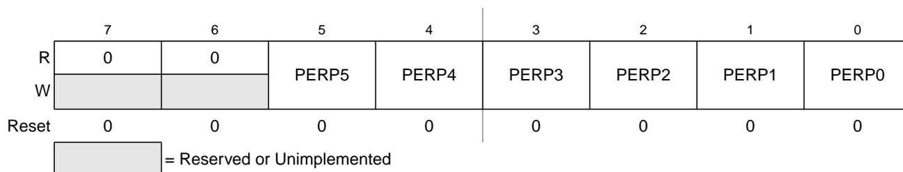
**Figure 3-21. Port P Pull Device Enable Register (PERP)**
