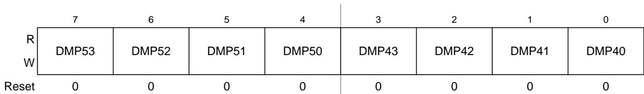
**Figure 11-14. PMF Disable Mapping C Register (PMFDMPC)**
