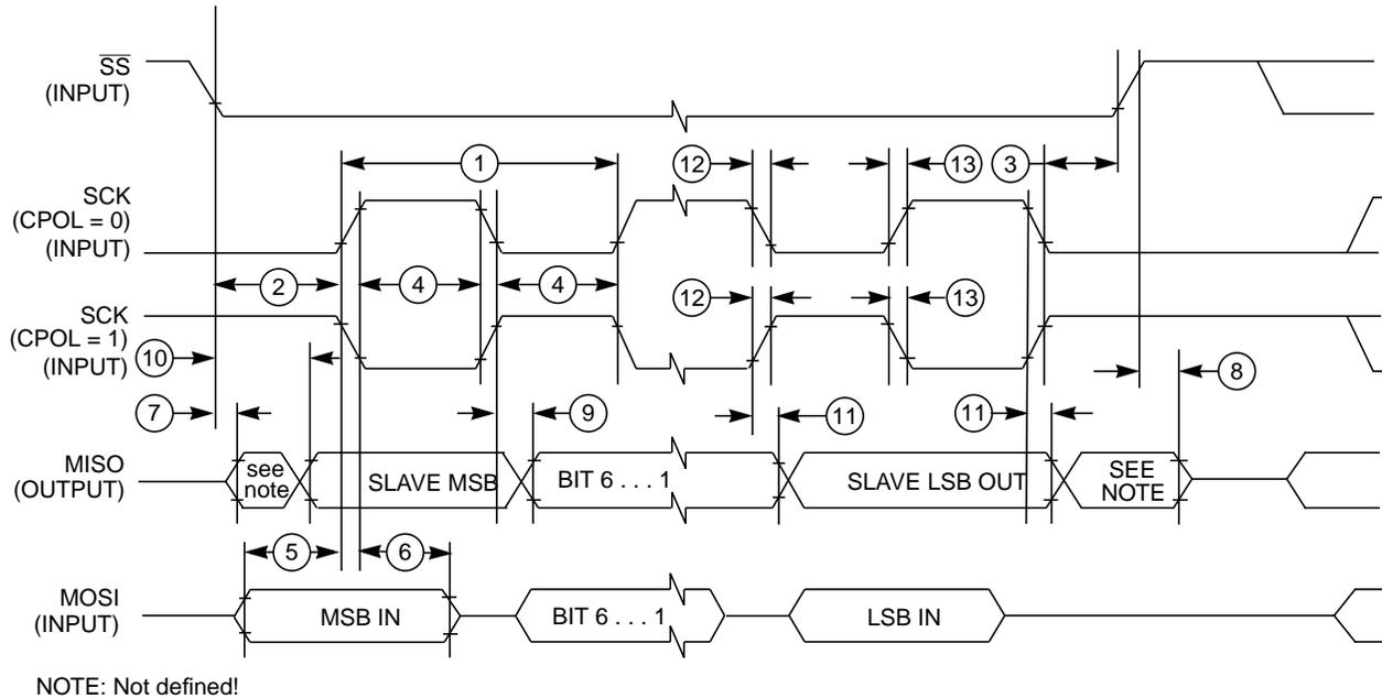
**Figure A-6. SPI Slave Timing (CPHA = 0)**
