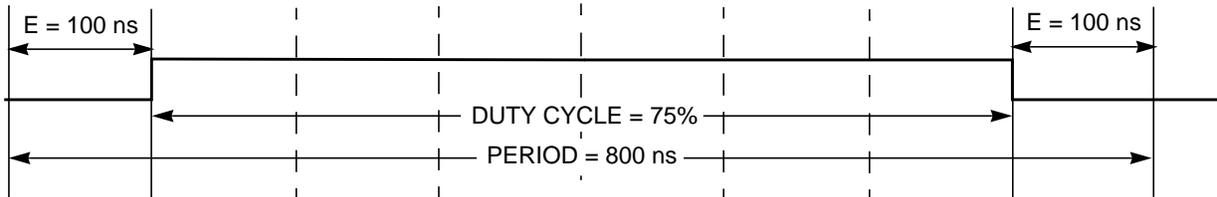
Figure 12-39. PWM Center Aligned Output Example Waveform
