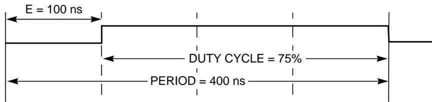
Figure 12-37. PWM Left Aligned Output Example Waveform
