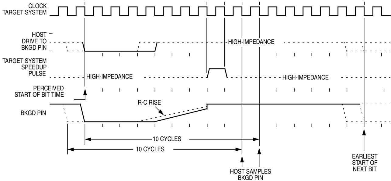
**Figure 15-8. BDM Target-to-Host Serial Bit Timing (Logic 1)**
