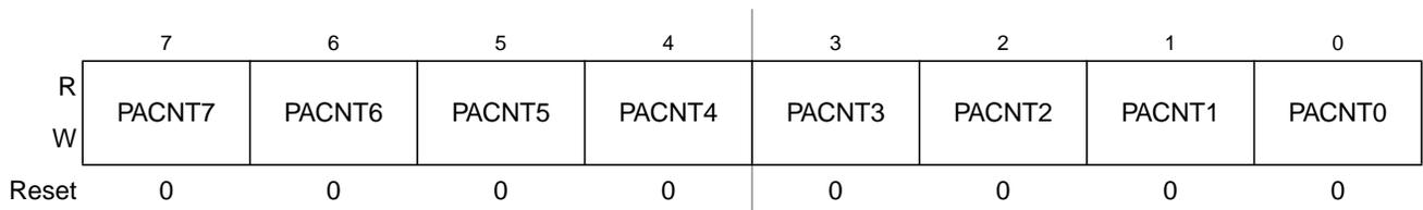
**Figure 13-25. Pulse Accumulator Count Register Low (PACNTL)**
