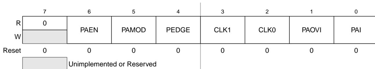
**Figure 13-22. 16-Bit Pulse Accumulator Control Register (PACTL)**
