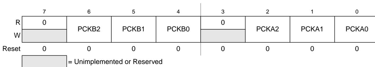
**Figure 12-6. PWM Prescaler Clock Select Register (PWMPRCLK)**
