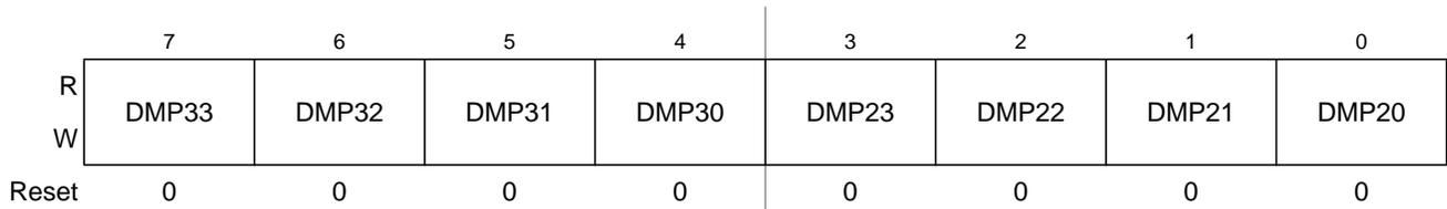
**Figure 11-13. PMF Disable Mapping B Register (PMFDMPB)**
