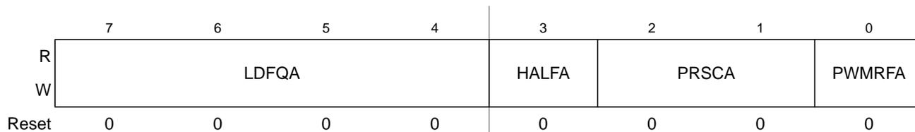
Figure 11-27. PMF Frequency Control A Register (PMFFQCA)
