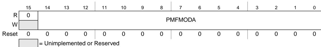
**Figure 11-29. PMF Counter Modulo A Register (PMFMODA)**
