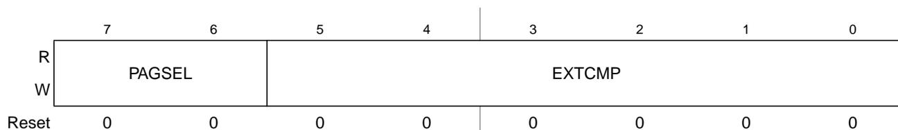
Figure 16-19. Debug Comparator B Extended Register (DBGCBX)
