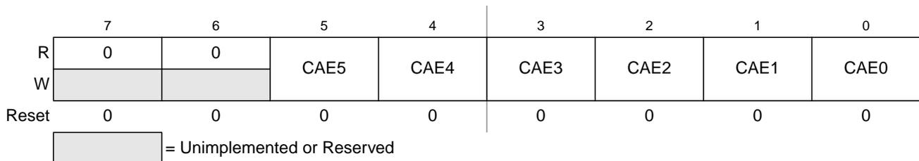
**Figure 12-7. PWM Center Align Enable Register (PWMCAE)**
