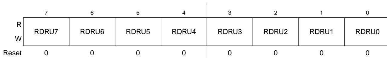
Figure 3-45. Port U Reduced Drive Register (RDRU)
