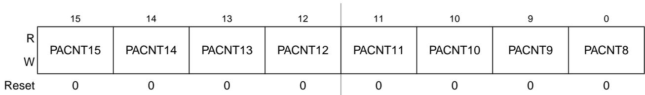
**Figure 13-24. Pulse Accumulator Count Register High (PACNTH)**
