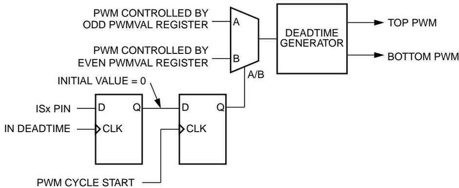
**Figure 11-57. Internal Correction Logic when ISENS = 10**
