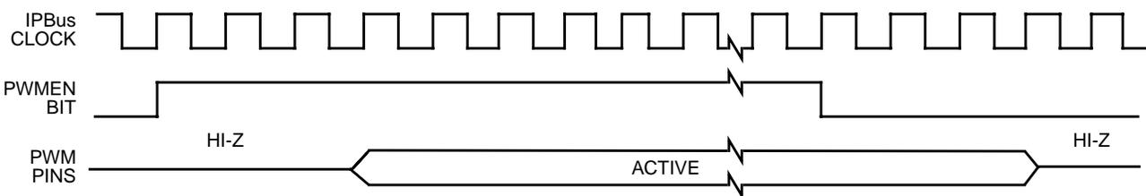
Figure 11-75. PWMEN and PWM Pins in Complementary Operation
