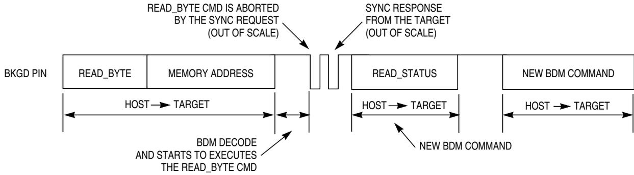
**Figure 15-12. ACK Abort Procedure at the Command Level**
