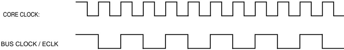
Figure 4-18. Core Clock and Bus Clock Relationship
