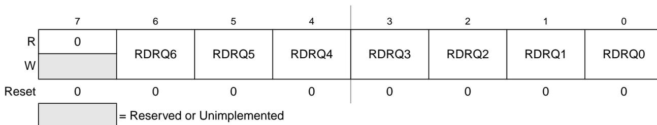
**Figure 3-26. Port Q Reduced Drive Register (RDRQ)**
