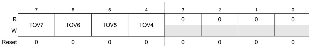
**Figure 13-13. Timer Toggle On Overflow Register 1 (TTOV)**
