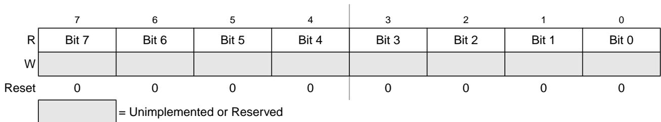
Figure 16-12. Debug Comparator C Register Low (DBGCCCL)
