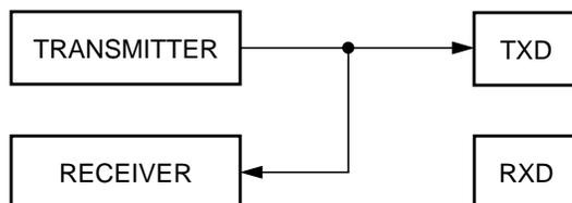
Figure 8-25. Loop Operation (LOOPS = 1, RSRC = 0)
