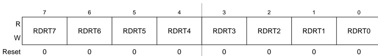
Figure 3-39. Port T Reduced Drive Register (RDRT)
