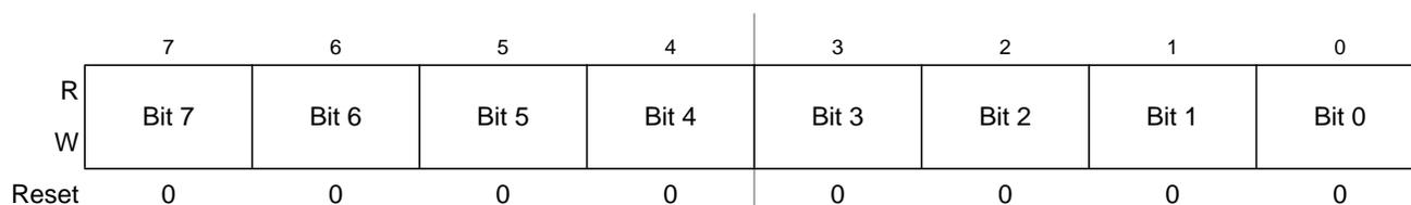
Figure 16-18. Debug Comparator A Register Low (DBGCAL)
