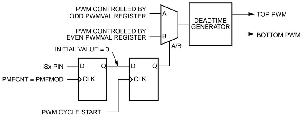
**Figure 11-58. Internal Correction Logic when ISENS = 11**
