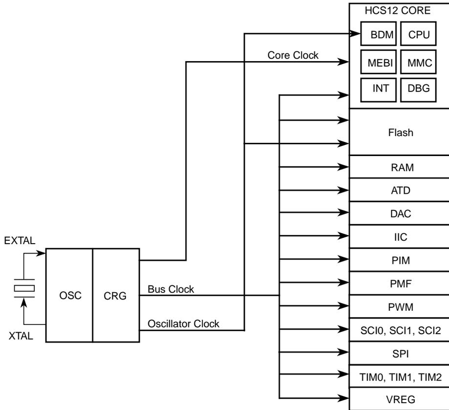
**Figure 1-10. Clock Connections**
