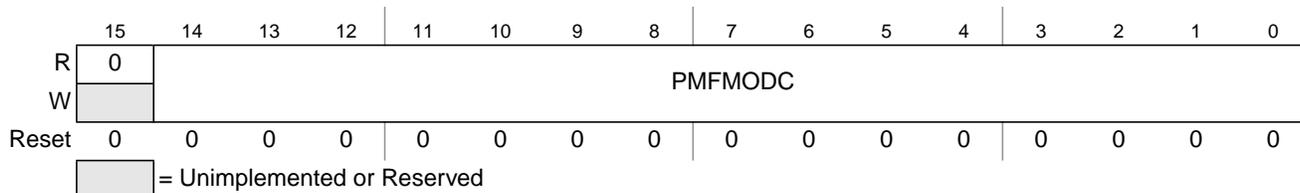
**Figure 11-39. PMF Counter Modulo C Register (PMFMODC)**
