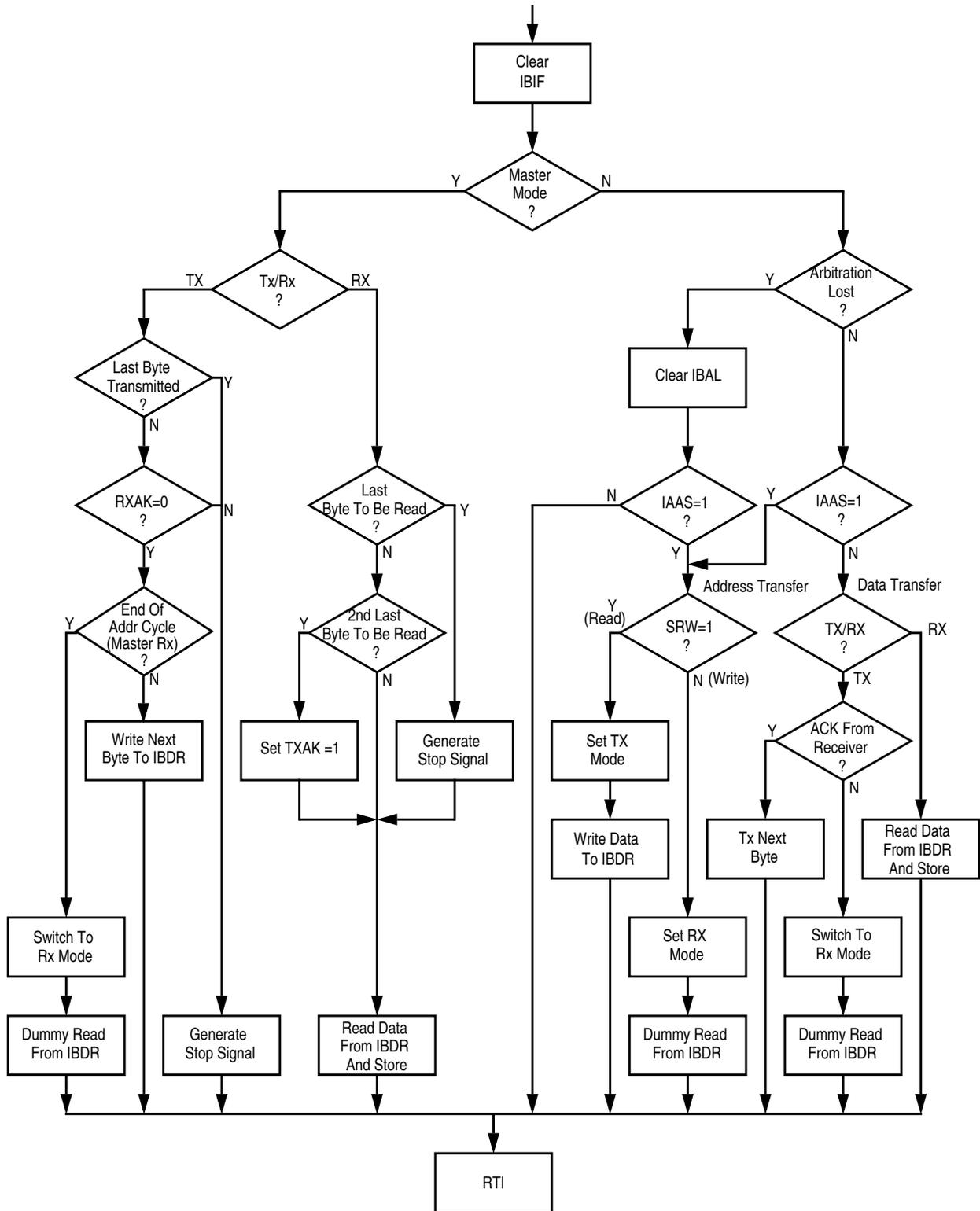
Figure 10-11. Flow-Chart of Typical IIC Interrupt Routine
