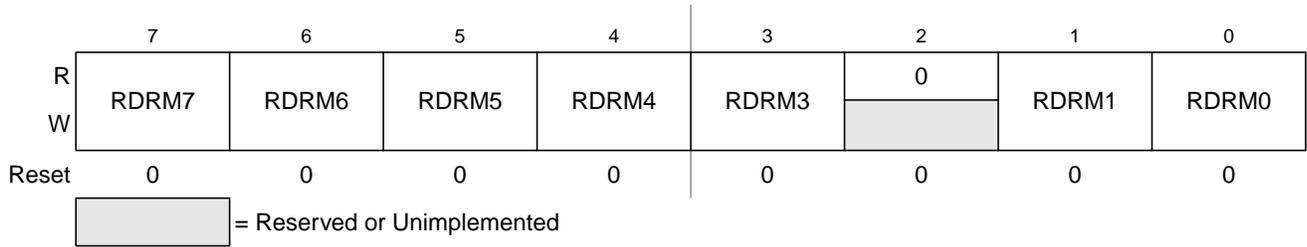
**Figure 3-13. Port M Reduced Drive Register (RDRM)**
