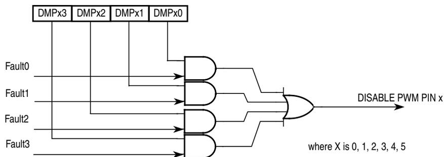
Figure 11-15. Fault Decoder
