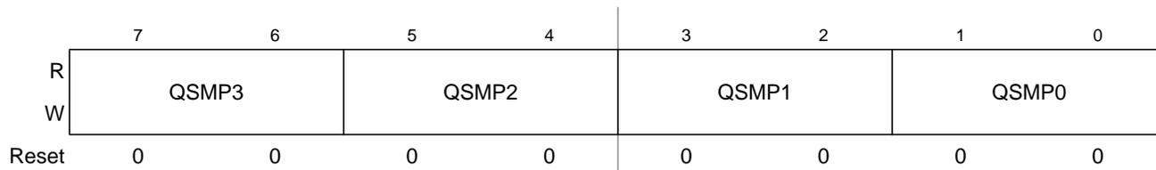
Figure 11-11. PMF Fault Qualifying Samples Register (PMFQSMP)
