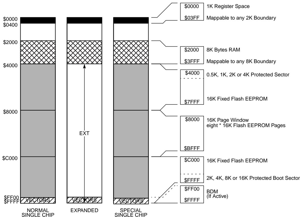
**Figure 1-2. MC9S12E128 User Configurable Memory Map**
