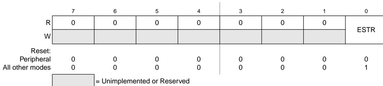
**Figure 18-16. External Bus Interface Control Register (EBICTL)**
