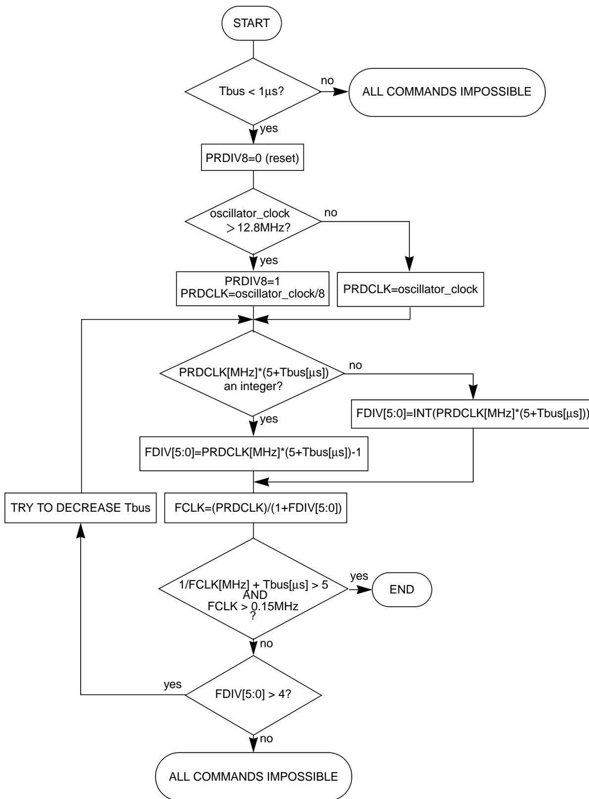
Figure 2-21. PRDIV8 and FDIV Bits Determination Procedure
