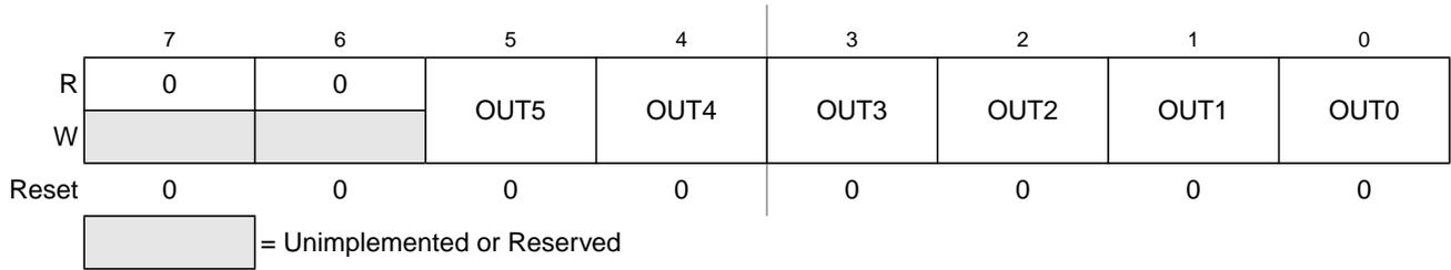
**Figure 11-17. PMF Output Control Bit Register (PMFOUTB)**
