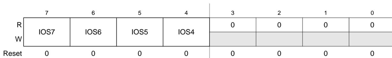
Figure 13-6. Timer Input Capture/Output Compare Select (TIOS)
