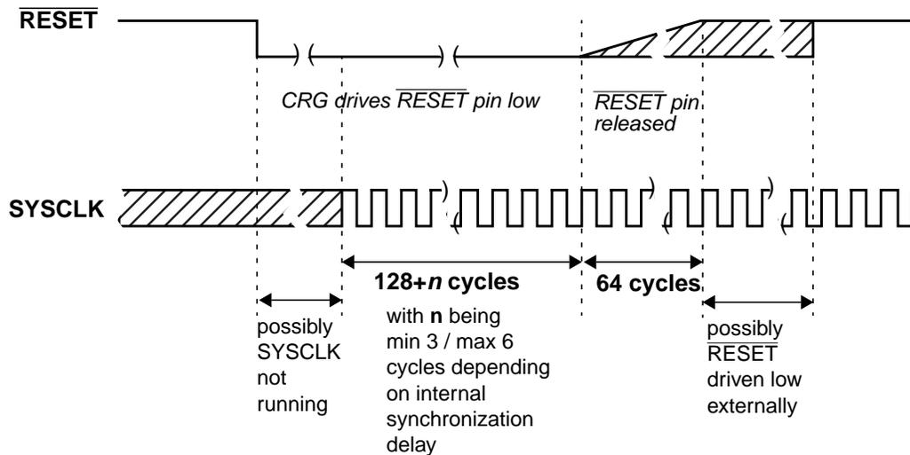
Figure 4-25.  $\overline{\text{RESET}}$  Timing
