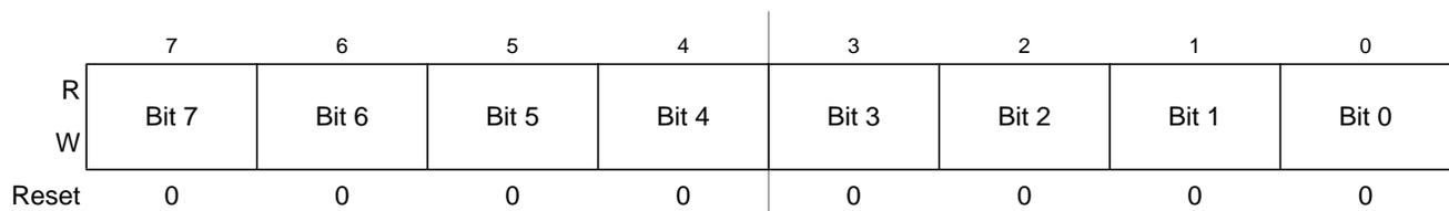
Figure 16-21. Debug Comparator B Register Low (DBGCBL)
