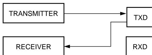
Figure 8-24. Single-Wire Operation (LOOPS = 1, RSRC = 1)
