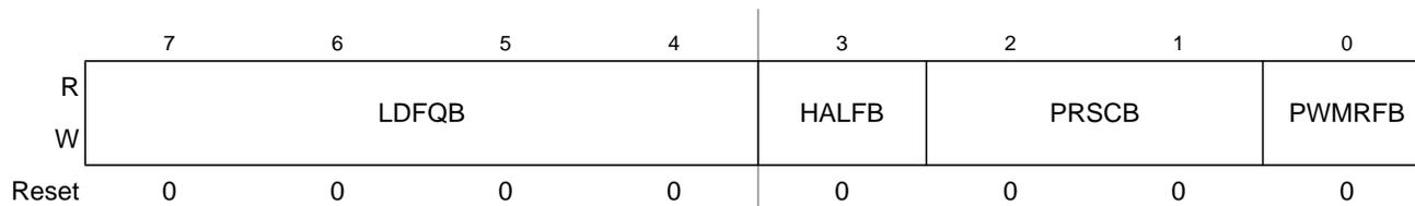
Figure 11-32. PMF Frequency Control B Register (PMFFQCB)
