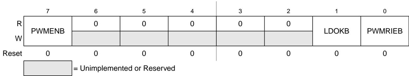
**Figure 11-31. PMF Enable Control B Register (PMFENCB)**
