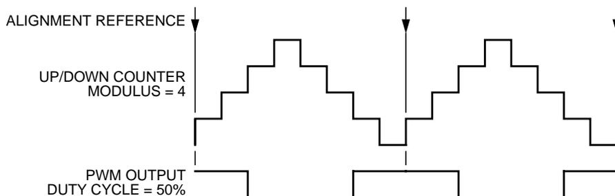
**Figure 11-41. Center-Aligned PWM Output**
