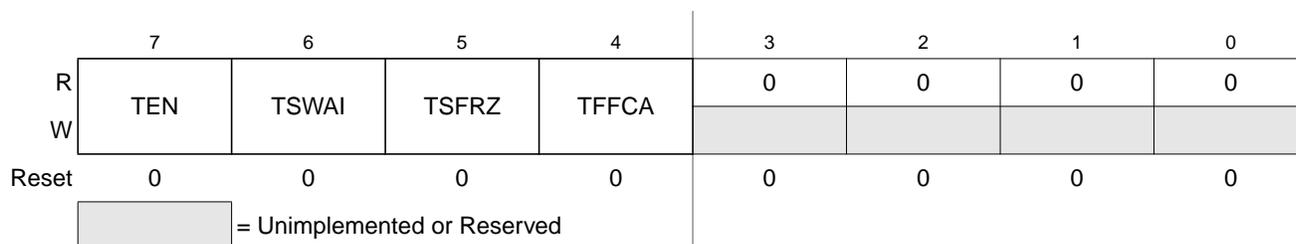
**Figure 13-12. Timer System Control Register 1 (TSCR2)**
