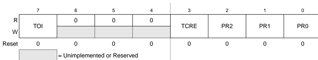
Figure 13-17. Timer System Control Register 2 (TSCR2)
