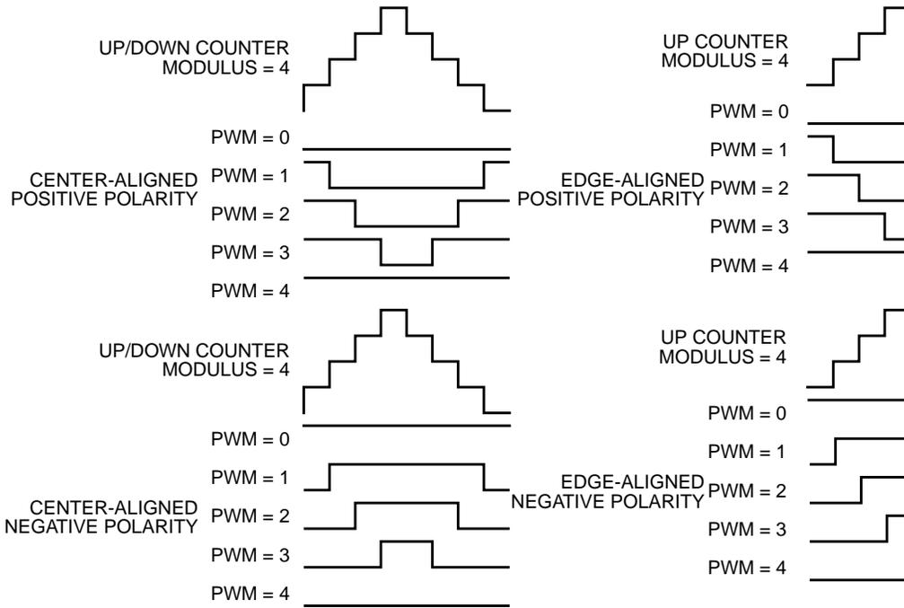
Figure 11-61. PWM Polarity
