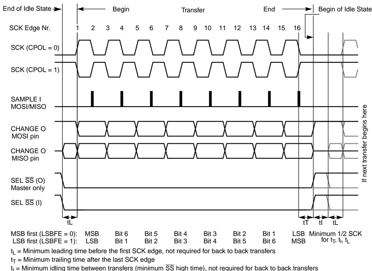
Figure 9-10. SPI Clock Format 1 (CPHA = 1)
