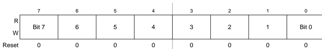
**Figure 18-20. Port K Data Direction Register (DDRK)**
