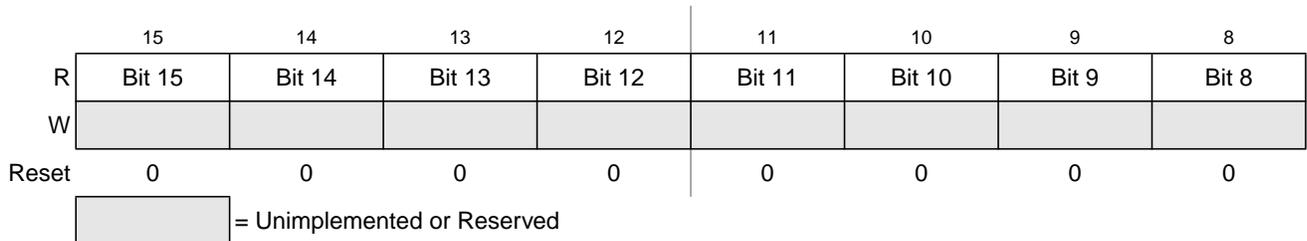
Figure 16-11. Debug Comparator C Register High (DBGCCCH)
