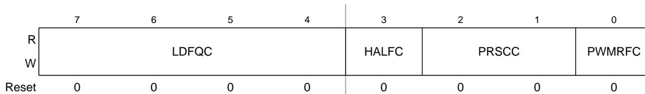
Figure 11-37. PMF Frequency Control C Register (PMFFQCC)
