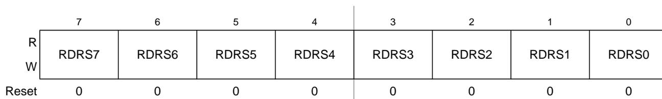
Figure 3-32. Port S Reduced Drive Register (RDRS)
