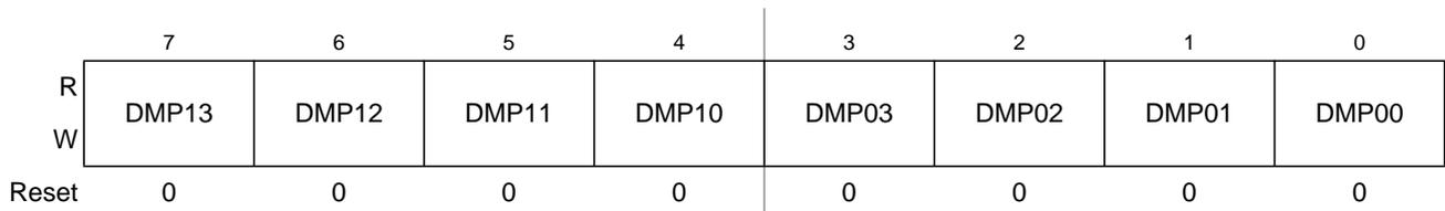
**Figure 11-12. PMF Disable Mapping A Register (PMFDMPA)**
