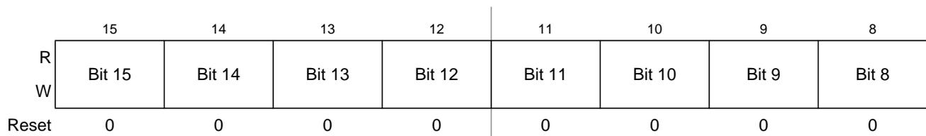
Figure 16-20. Debug Comparator B Register High (DBGCBH)
