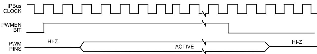
Figure 11-74. PWMEN and PWM Pins in Independent Operation
