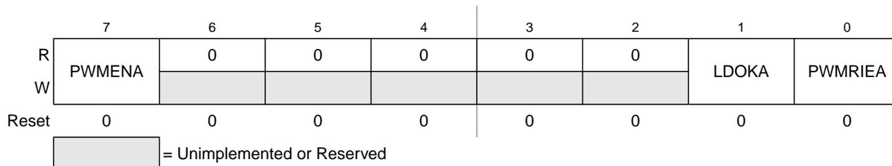
**Figure 11-26. PMF Enable Control A Register (PMFENCA)**
