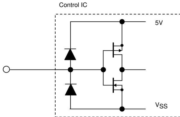
All input pins of this driver support schmitt input. Typ specifications at  $T_c = 25^\circ\text{C}$  are given below. Hysteresis voltage is 0.6V ( $V_{IHa} - V_{ILa}$ ).
