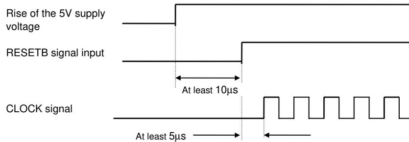
Figure 1 RESETB and CLOCK Signals Input Timing
