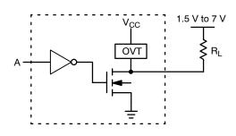
Figure 6. Output Voltage Mismatch Application
