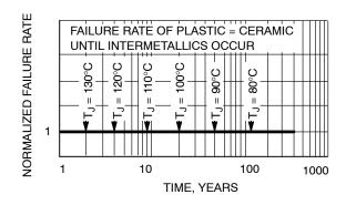
Figure 3. Failure Rate vs. Time Junction Temperature
