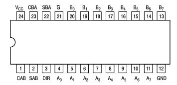
Figure 5. Pinout: 24-Lead Packages Conductors (Top View)
