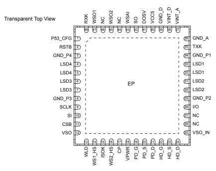
Figure 3. SB0400 48-pin QFN-EP pinout diagram
