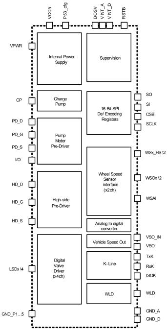
Figure 2. SB0400 simplified block diagram
