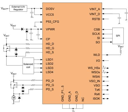
Figure 1. SB0400 simplified application diagram
