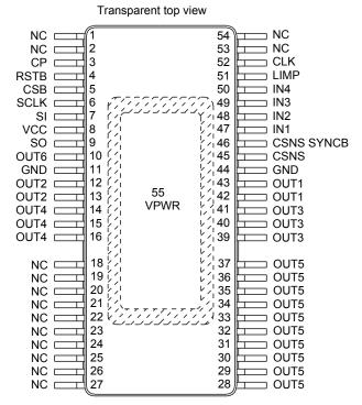
Figure 4. Pinout diagram for 54 pin SOIC-EP Package
