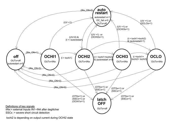
Figure 15. Output control diagram in fail mode
