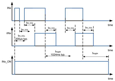
Figure 36. IN, iIN and IN\_ON signal
