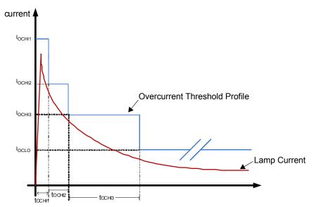
Figure 16. Transient overcurrent profile
