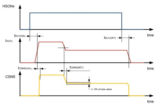
Figure 28. Current sensing response time
