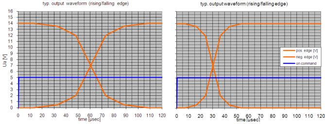
Figure 11. Typical power output switching (slow and fast slew rate)
