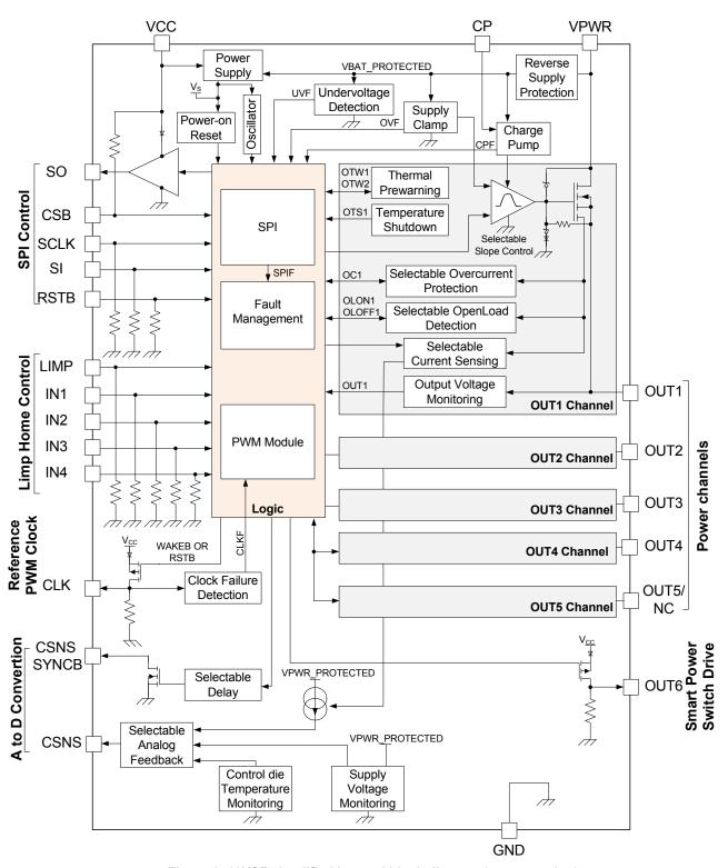
Figure 2. 12XSF simplified internal block diagram (penta version)
