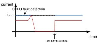
Figure 19. Overcurrent level fixed to OCLO
