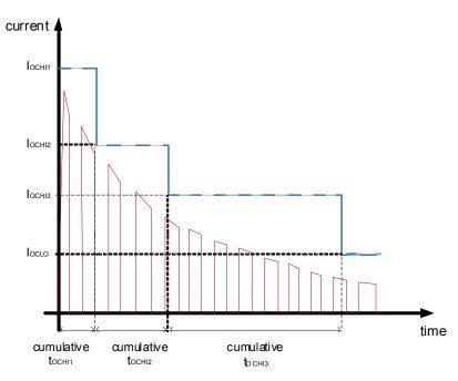
Figure 17. Transient overcurrent profile in PWM mode
