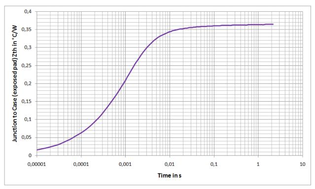
Figure 39. Transient thermal response curve
