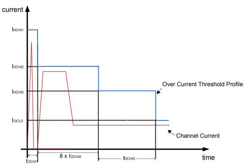
Figure 20. HID ballast overcurrent profile
