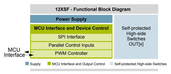
Figure 7. Functional block diagram
