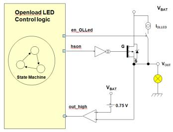
Figure 23. Open load in on state diagram for LED
