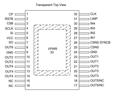
Figure 3. Pinout diagram for 32 pin SOIC-EP package
