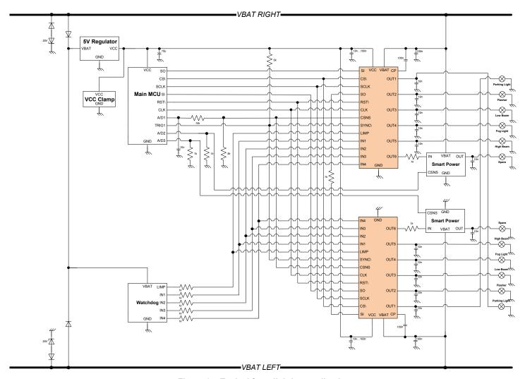
Figure 37. Typical front lighting application
