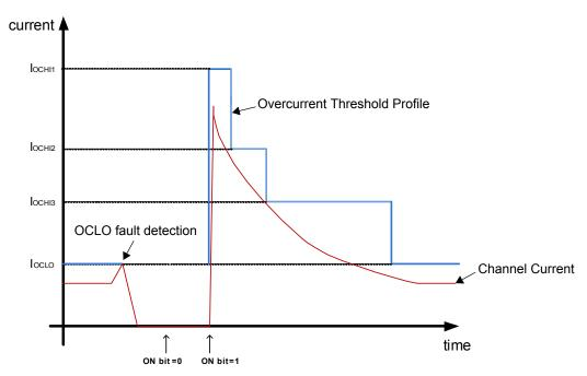
Figure 18. Resetable overcurrent profile
