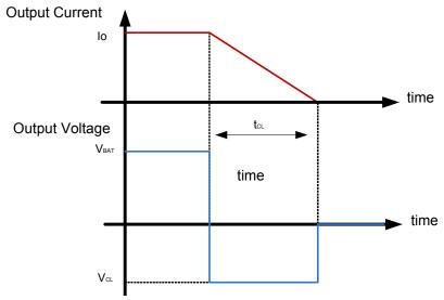
Figure 22. Simplified negative output clamp waveform
