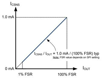
Figure 27. Output current sensing
