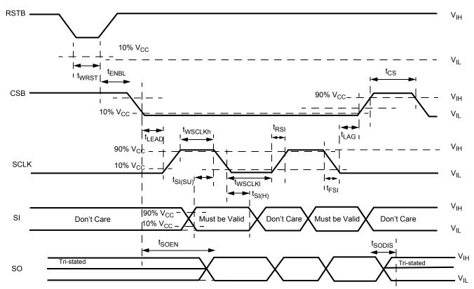
Figure 9. Timing requirements during SPI communication
