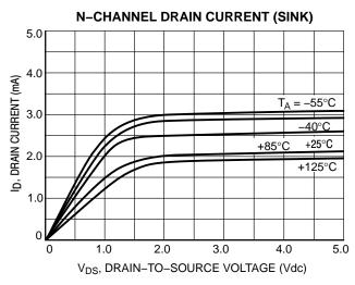
Figure 5.  $V_{GS} = 5.0 \text{ Vdc}$
