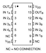
Figure 1. Pin Assignment
