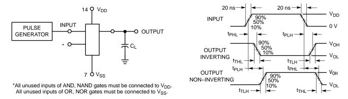
Figure 3. Switching Time Test Circuit and Waveforms
