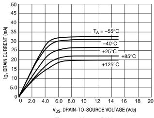
Figure 9.  $V_{GS} = 15 \text{ Vdc}$
