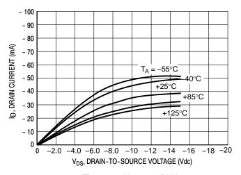
Figure 10.  $V_{GS} = -15 \text{ Vdc}$
