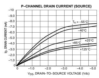
Figure 6.  $V_{GS} = -5.0 \text{ Vdc}$
