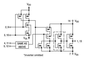
Figure 4. Circuit Schematic - One of Two Gates Shown
