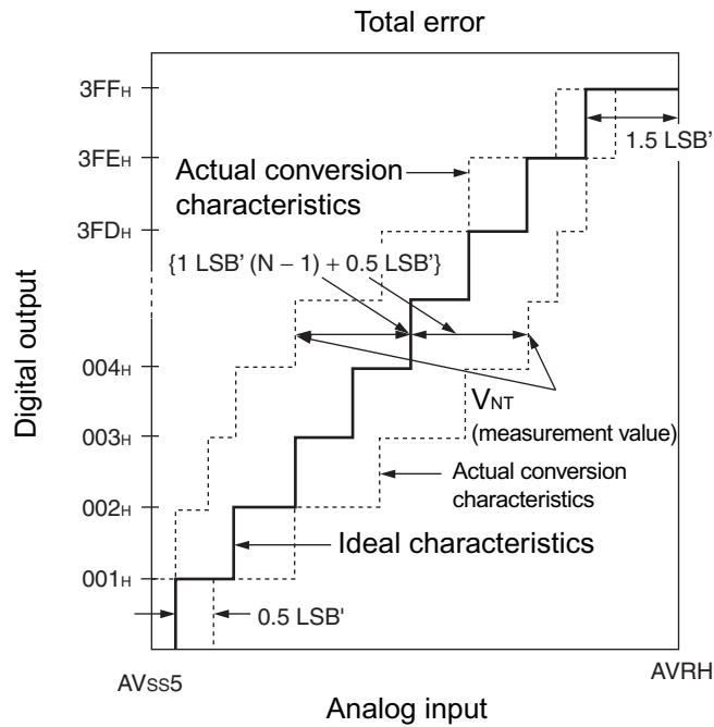
$$1\text{LSB}' \text{ (ideal value)} = \frac{\text{AVRH} - \text{AV}_{\text{ss}5}}{1024} \text{ [V]}$$
