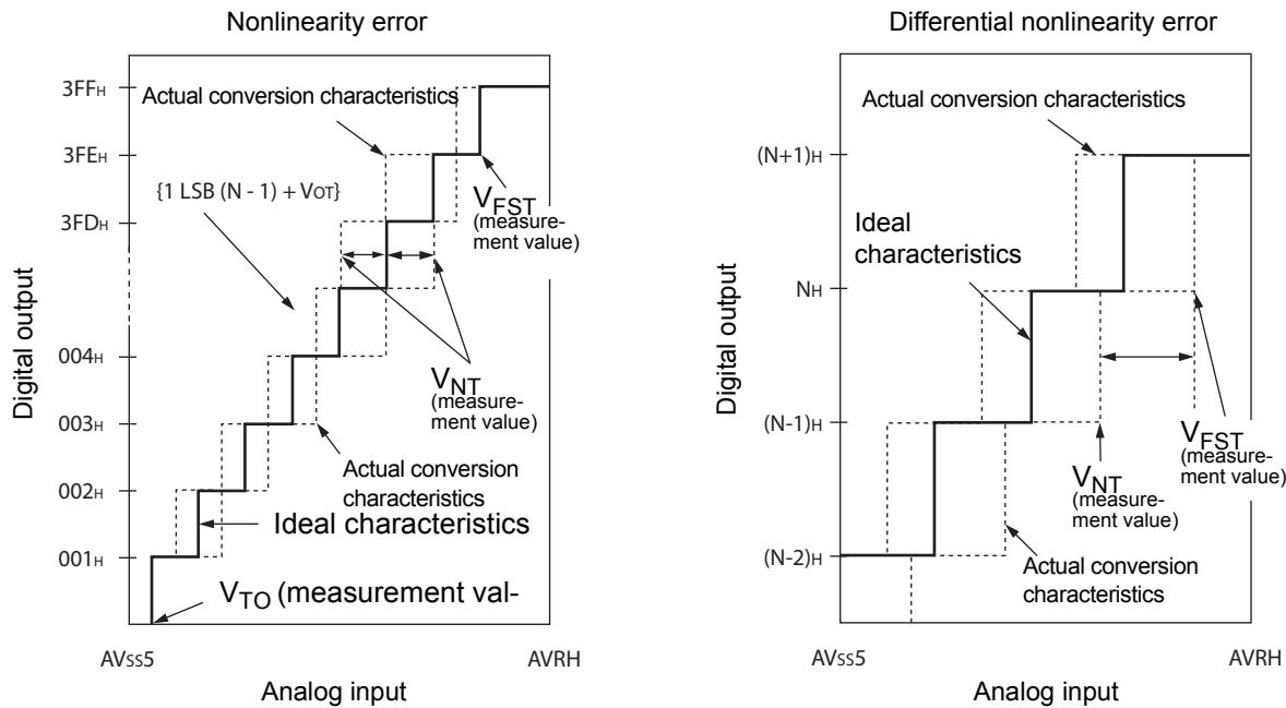
$$\text{Nonlinearity error of digital output } N = \frac{V_{NT} - \{1\text{LSB} \cdot (N - 1) + V_{OT}\}}{1\text{LSB}} \quad [\text{LSB}]$$
