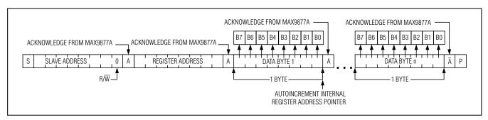
Figure 10. Writing n-Bytes of Data to the MAX9877A
