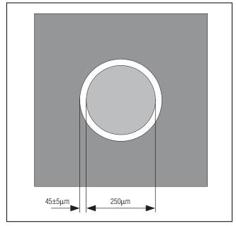
Figure 15. PCB Footprint Recommendation Diagram
