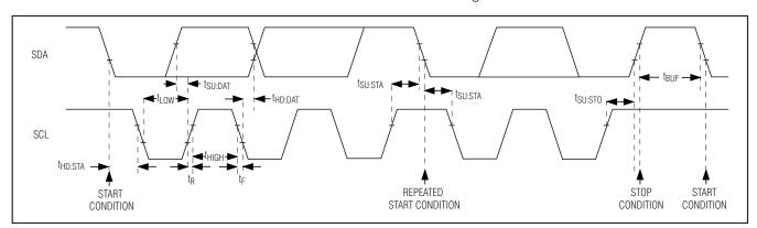
Figure 6. 2-Wire Interface Timing Diagram
