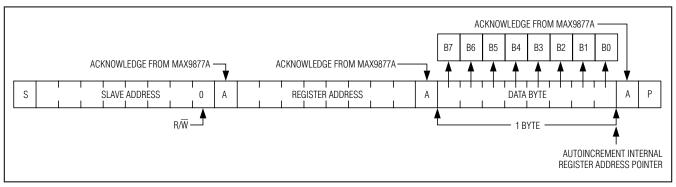
Figure 9. Writing One Byte of Data to the MAX9877A
