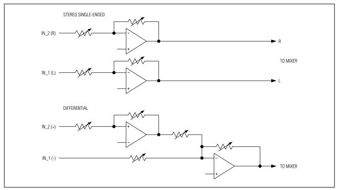
Figure 2. Differential and Stereo Single-Ended Input Configurations
