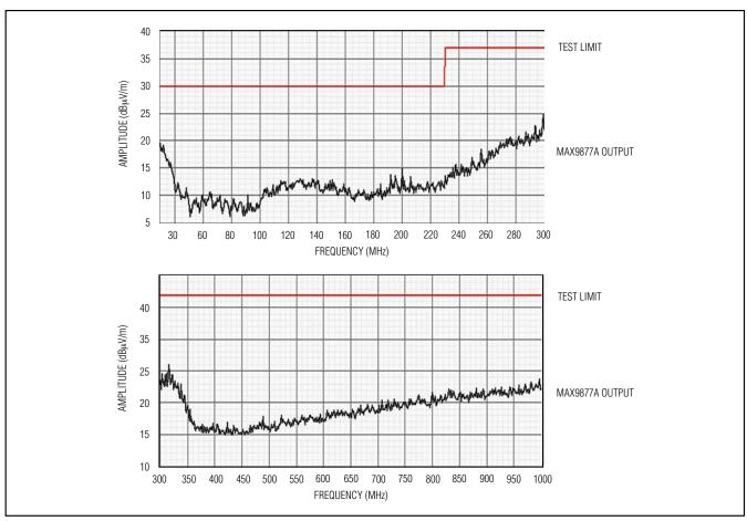
Figure 4. EMI with 152mm of Speaker Cable
