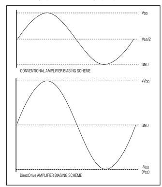
Figure 5. Traditional Amplifier Output vs. MAX9877A DirectDrive Output
