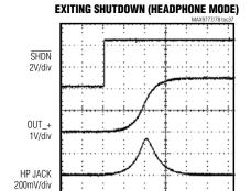
$\begin{array}{c} \text{100ms/div} \\ \text{R}_{L} = 16\Omega \\ \text{INPUT AC-COUPLED TO GND} \end{array}$
