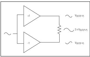
Figure 8. Bridge-Tied Load Configuration
