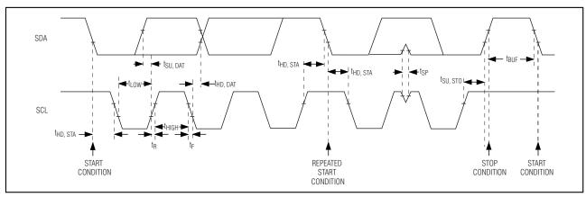
Figure 3. 2-Wire Serial-Interface Timing Diagram
