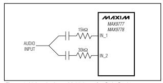
Figure 1. Using the Input Multiplexer for Gain Setting
