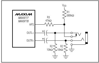
Figure 2. HPS Configuration Circuit
