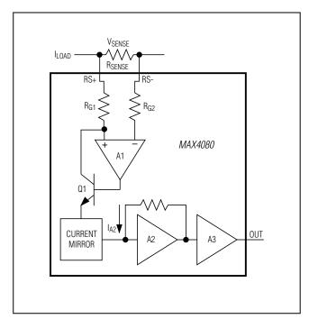
Figure 2. MAX4080 Functional Diagram
