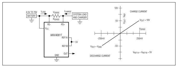
Figure 1. MAX4081T OUT Transfer Curve
