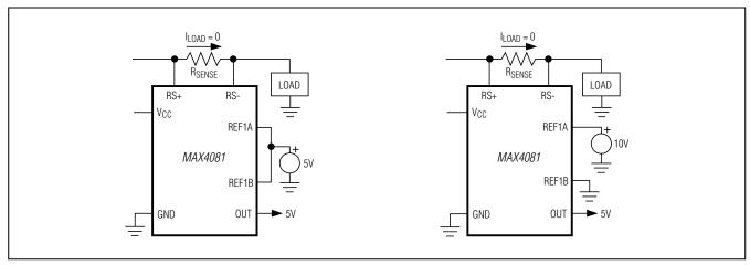
Figure 4. MAX4081 Reference Inputs
