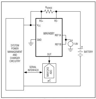
Figure 5. MAX4081 Used In Smart-Battery Application
