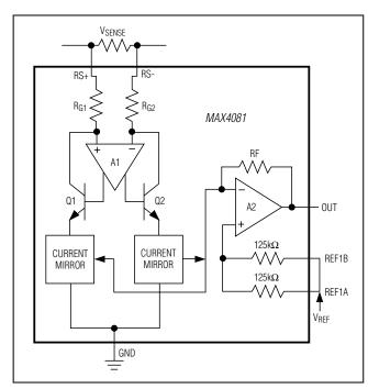
Figure 3. MAX4081 Functional Diagram
