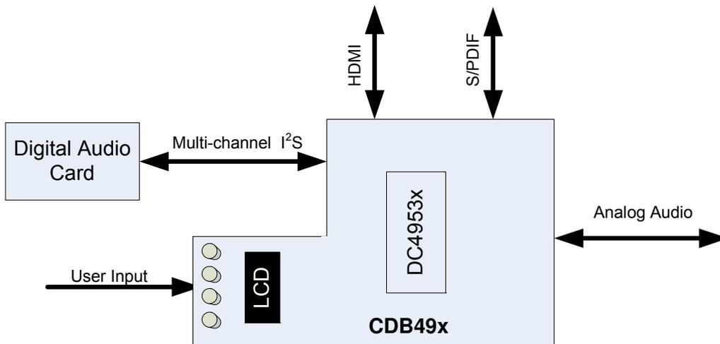
Figure 2-2. CK49x System Block Diagram in Standalone Mode
