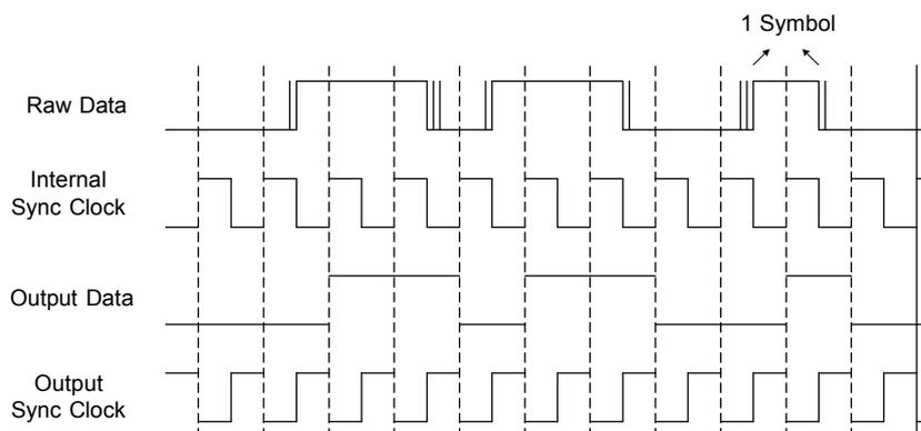
**Figure 21. Demodulated Data and Sync Clock Timing Characteristics**
