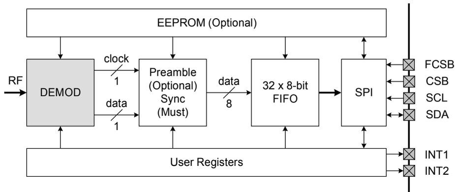
Figure 22. Data Path of Buffer Mode
