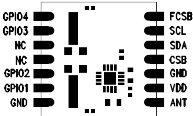
Figure 2. Pin Diagram
