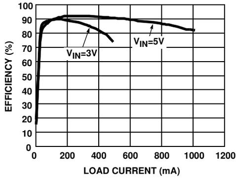
FIGURE 1. BOOST EFFICIENCY AT  $V_{OUT} = 12V$  (PI MODE)
