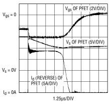
TEST PERFORMED ON DEMOBOARD V<sub>CHARGE</sub> = 12.6V  $V_{IN} = 15VDC$ CHARGER = ON PFET = 1/2 Si4925DY I<sub>CHARGE</sub> = <10mA
