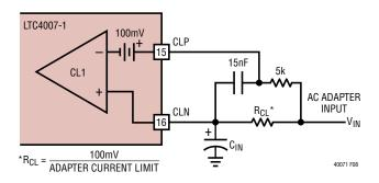
Figure 8. Adapter Current Limiting
