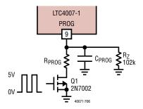
Figure 6. PWM Current Programming
