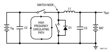
Figure 12. High Speed Switching Path
