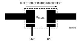
Figure 13. Kelvin Sensing of Charging Current
