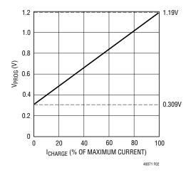
Figure 2. V<sub>PROG</sub> vs I<sub>CHARGE</sub>
