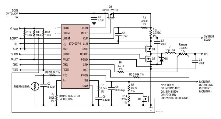
Figure 11. Circuit Application (16.8V/3A) to Automatically Trickle Charge Depleted Batteries
