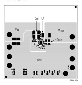
Figure 3a. Sample PCB Layout—Topside
