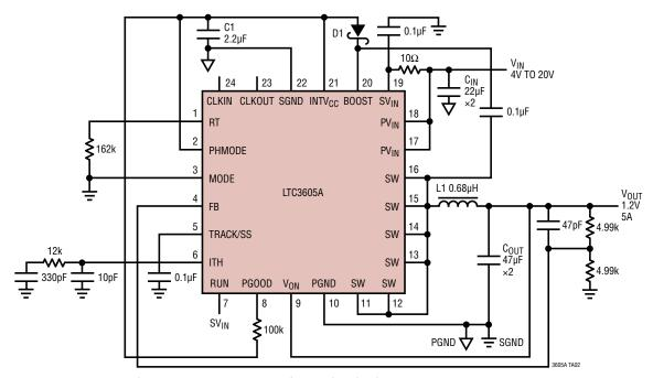
C1: AVX 0805ZD225MAT2A C<sub>IN</sub>: TDK C4532X5RIC226M C<sub>OUT</sub>: TDK C3216X5ROJ476M D1: CENTRAL SEMI CMDSH-3 L1: VISHAY IHLP-2525CZERR68-M01
