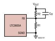
Figure 1. Setting the Output Voltage
