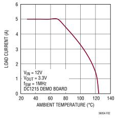
Figure 2. Load Current vs Ambient Temperature
