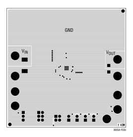
Figure 3b. Sample PCB Layout—Bottom Side
