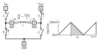
Figure 4. Inductor Disharge Cycle During Burst Mode Operation
