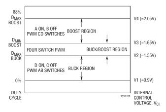
Figure 2. Switch Control vs Internal Control Voltage, V<sub>CI</sub>
