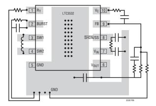
Figure 6. Recommended Component Placement. Traces Carrying High Current are Direct. Trace area at FB and  $V_{\mathbb{C}}$  Pins are Kept Low. Lead Length to Battery Should be Kept Short
