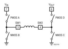
Figure 1. Simplified Diagram of Output Switches
