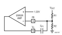
Figure 7. Error Amplifier with Type I Compensation
