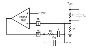
Figure 8. Error Amplifier with Type III Compensation
