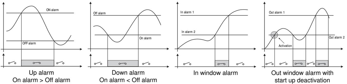
**Note:** any alarm working mode can be linked to the “start up deactivation” function which disables only the first alarm after power on of the transducer.
