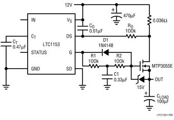
Figure 3. Powering Large Capacitive Loads
