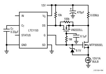
Figure 4. Lamp Driver with Delayed Protection
