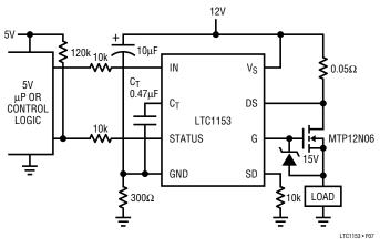
Figure 7. Reverse Battery Protection
