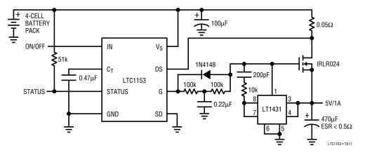
"4 Cell-to-5V" Regulator with 2A Current Limit, Auto-Reset, Ramped Turn-On and 10μA Standby Current
