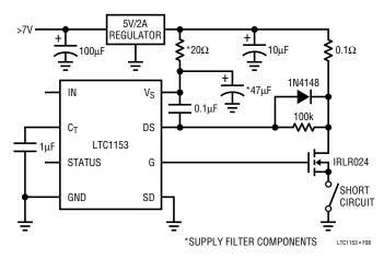
Figure 8. Supply Filter for Current Limited Supplies
