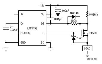
Figure 6. Using a Speed-Up Diode
