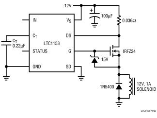
Figure 2. Protecting Inductive Loads
