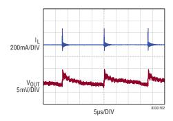
Figure 2. Burst Mode Operation
