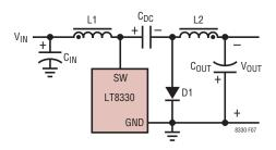
Figure 7. A Simplified Inverting Converter
