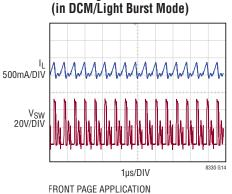
$V_{IN} = 12V$ ,  $V_{OUT} = 48V$ ,  $I_{LOAD} = 20mA$
