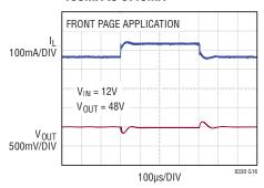
V<sub>OUT</sub> Transient Response: Load Current Transients from 5mA to 135mA to 5mA
