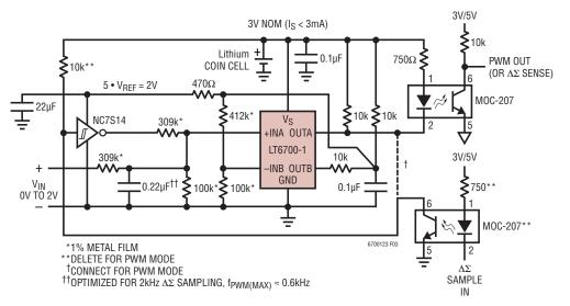
Figure 3. Isolated PWM or  $\Delta\Sigma$  Converter
