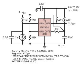
Figure 2. Micropower Thermostat/Temperature Alarm
