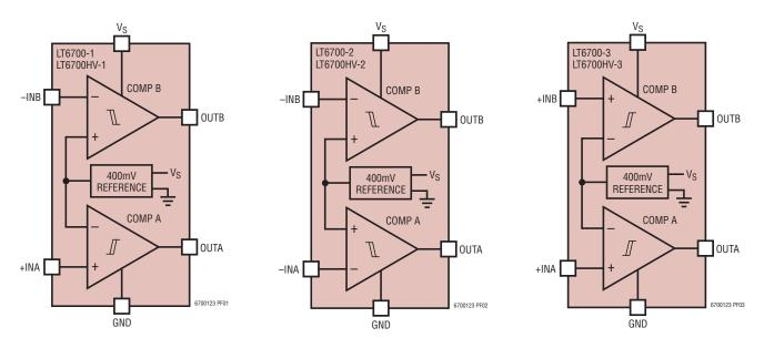
**OUTA:** Open-Collector Output of Comparator Section A. This pin provides drive for up to 40mA of load current. Offstate voltage may be as high as 18V (36V for LT6700HV) above GND, regardless of  $V_S$  used.
