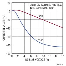
Figure 3. Ceramic Capacitor DC Bias Characteristics
