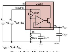
Figure 1. Basic Adjustable Regulator
