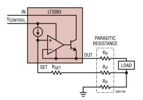
Figure 6. Connections for Best Load Regulation
