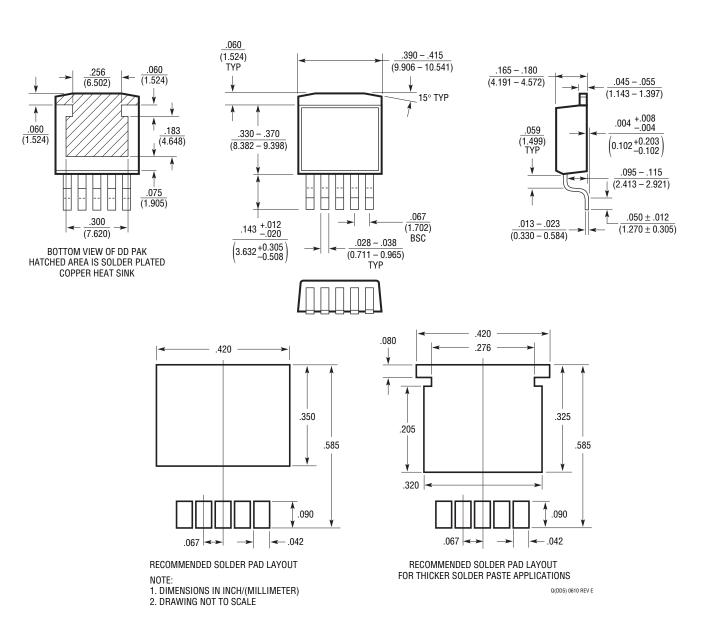
Q Package 5-Lead Plastic DD-PAK (Reference LTC DWG # 05-08-1461 Rev E)
