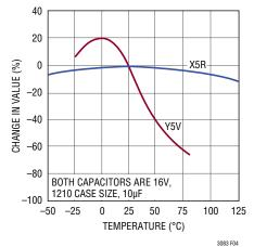
Figure 4. Ceramic Capacitor Temperature Characteristics
