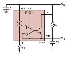
Figure 8. Reducing Power Dissipation Using a Parallel Resistor
