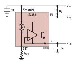
Figure 7. Reducing Power Dissipation Using a Series Resistor
