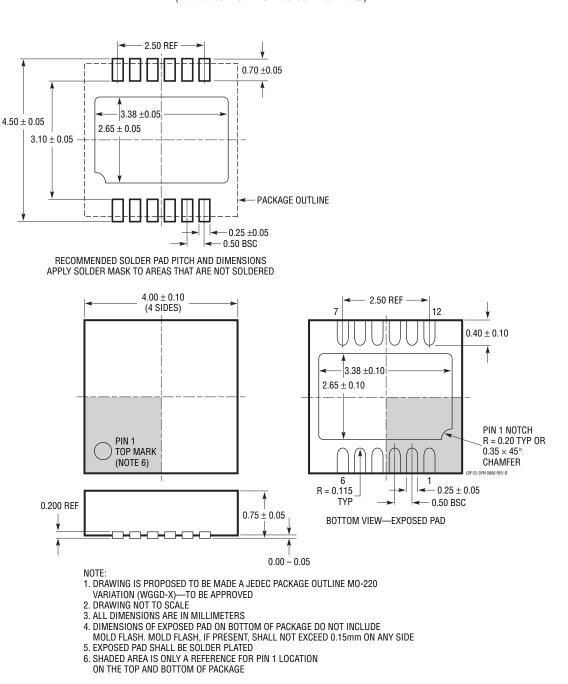
DF Package 12-Lead Plastic DFN (4mm × 4mm) (Reference LTC DWG # 05-08-1733 Rev Ø)
