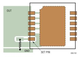
Figure 2. Guard Ring Layout Example for DF Package
