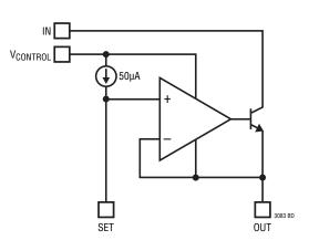
The LT3083 regulator is easy to use and has all the protection features expected in high performance regulators. Included are short-circuit protection and safe operating area protection, as well as thermal shutdown with hysteresis.
